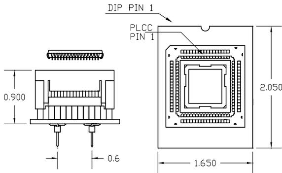
Press rim to open socket, press device to close
