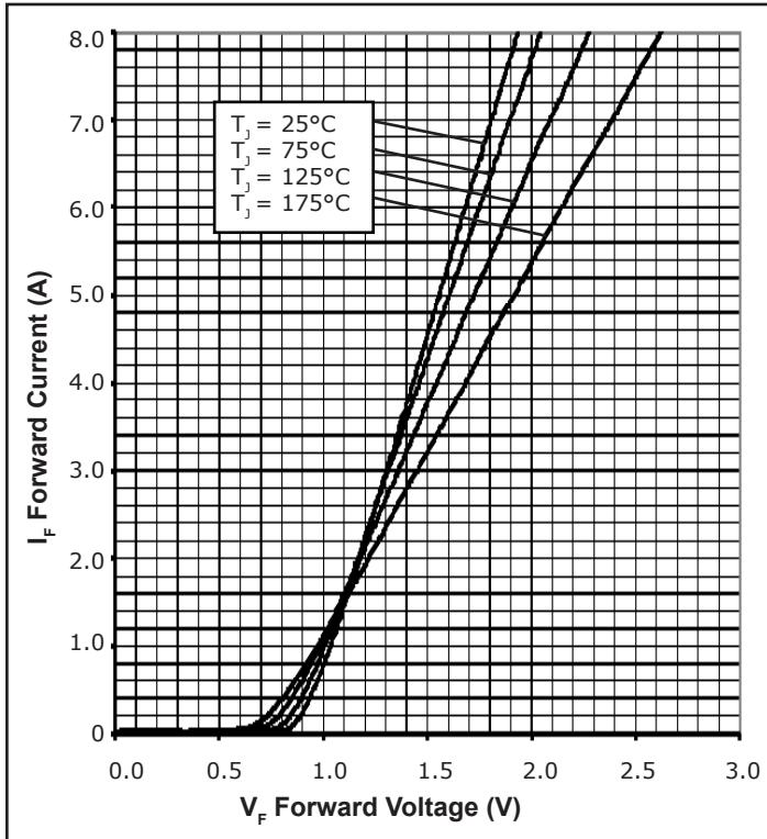
Figure 1. Forward Characteristics
