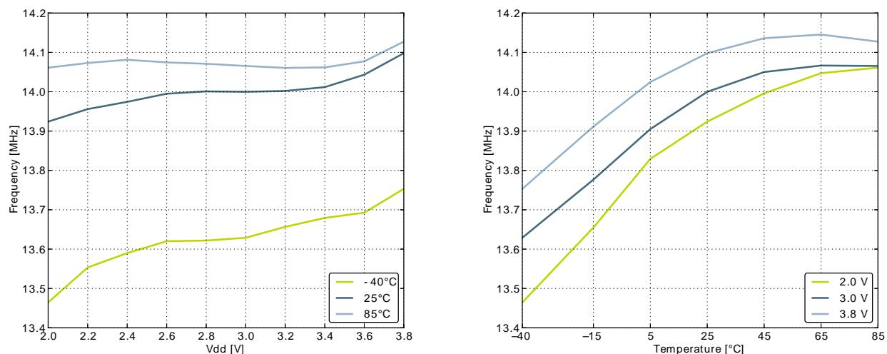
**Figure 3.15. Calibrated HFRCO 21 MHz Band Frequency vs Supply Voltage and Temperature**
