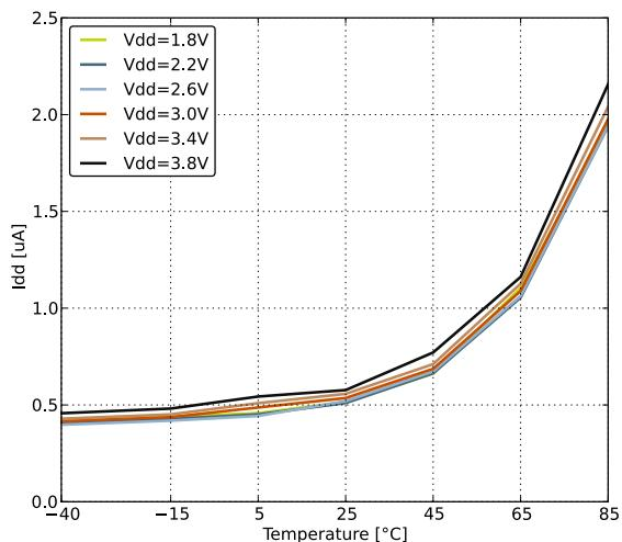
**Figure 3.3.** EM4 current consumption.
