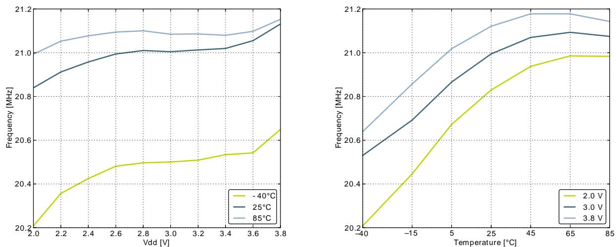
**Figure 3.16. Calibrated HFRCO 28 MHz Band Frequency vs Supply Voltage and Temperature**
