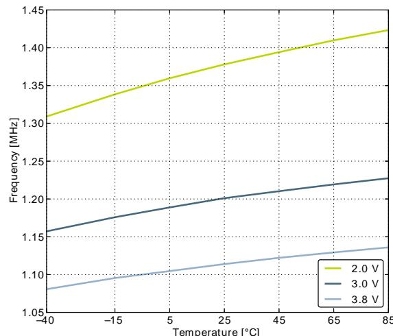
**Figure 3.12. Calibrated HFRCO 7 MHz Band Frequency vs Supply Voltage and Temperature**
