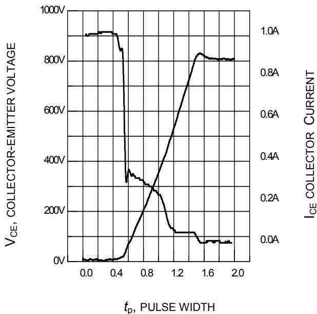
**Figure 21. Typical turn off behavior, soft switching**
