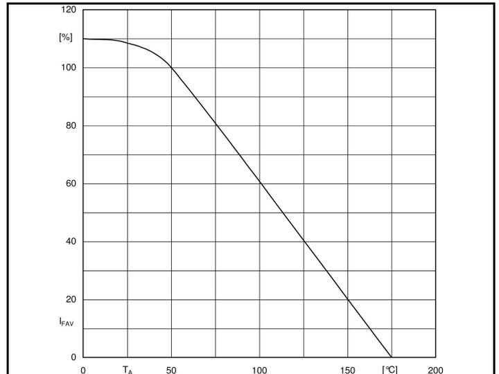
Fig. 2 Rated forward current vs. ambient temperature <sup>1)</sup>
