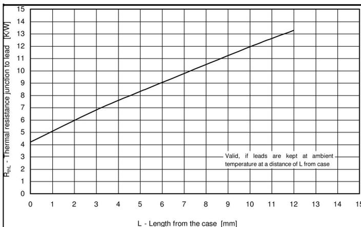
Fig. 5 Thermal resistance versus length from case
