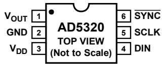
Figure 3. SOT-23 Pin Configuration
