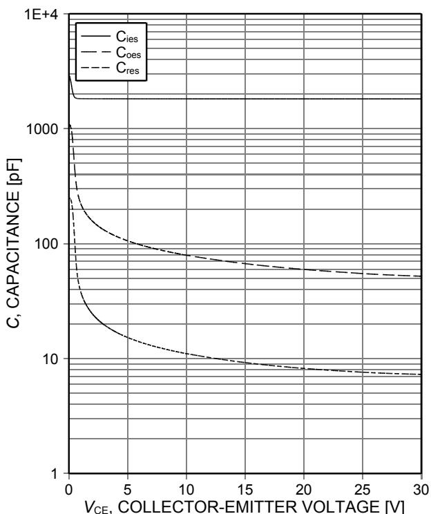
Figure 16. **Typical capacitance as a function of collector-emitter voltage**
