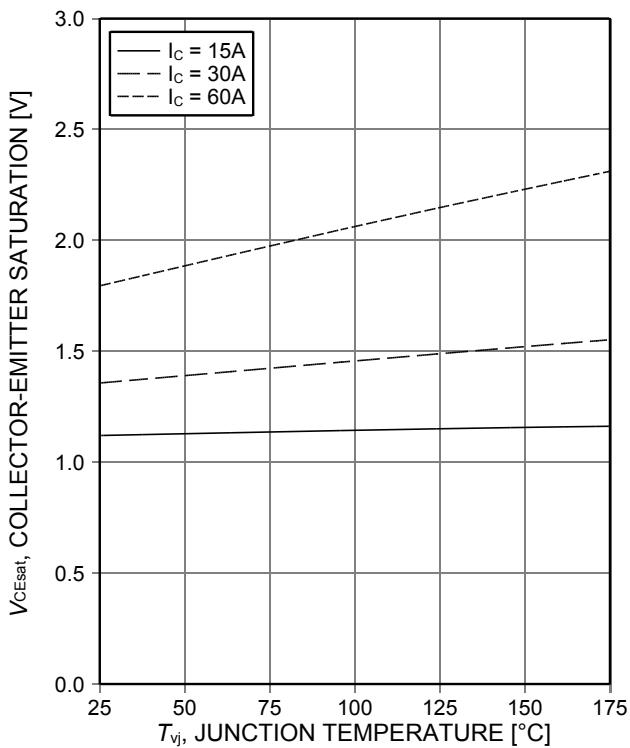
Figure 6. Typical collector-emitter saturation voltage as a function of junction temperature
