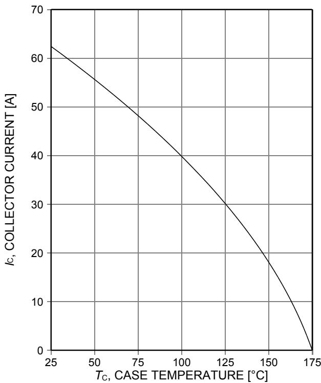
Figure 2. Collector current as a function of case temperature
