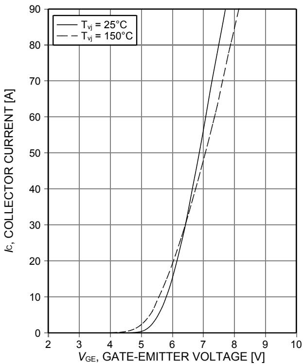
Figure 5. Typical transfer characteristic
