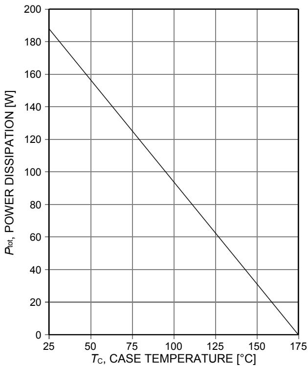
Figure 1. Power dissipation as a function of case temperature
