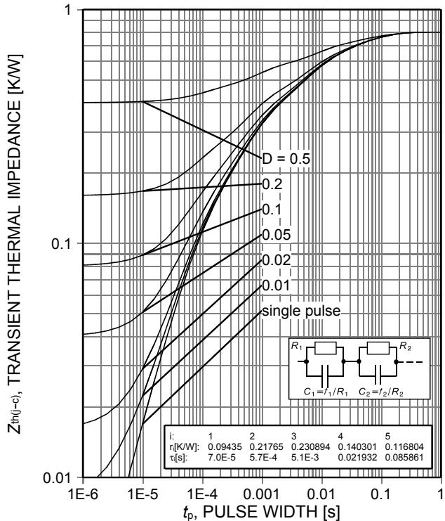
Figure 17. IGBT transient thermal impedance
