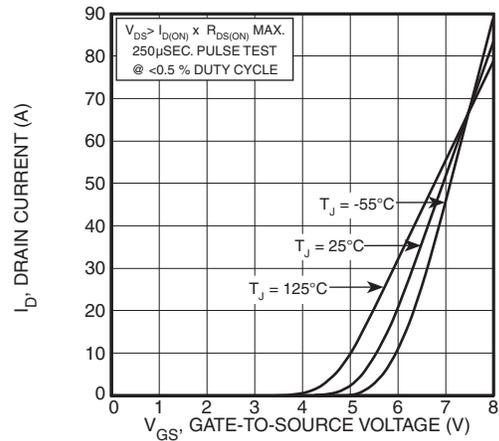
Figure 4, Transfer Characteristics
