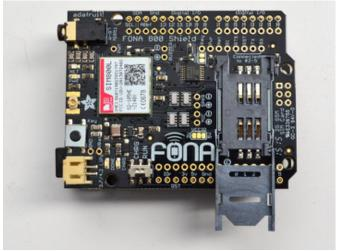
Open by sliding the cover towards the bottom of the shield
