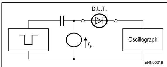
Pulse generator:  $t_p = 100\text{ns}$ ,  $D = 0.05$ ,  $t_r = 0.6\text{ns}$ ,
