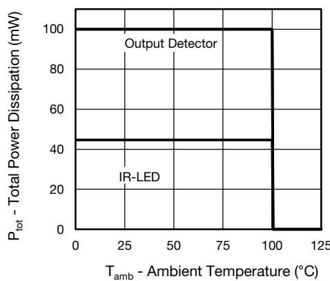
Fig. 1 - Maximum Power vs. Operating Temperature
