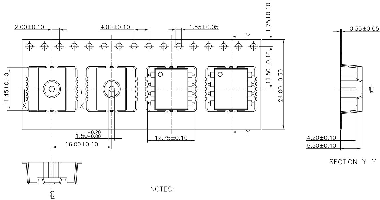
Fig. 16 - Tape and Reel Packing Option 7 (750 parts per reel)
