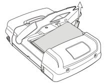
Figure 49. Removing the Battery
