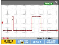
Figure 33. Triggering on Narrow Glitches
