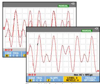
Figure 31. N-Cycle triggering
