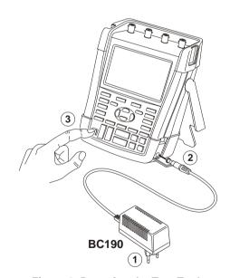
Figure 2. Powering the Test Tool
