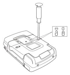
Figure 47. Unlocking the Battery Cover
