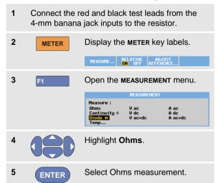
The resistor value is displayed in ohms. Observe also that the bargraph is displayed. (See 15.)
