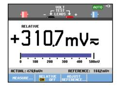
Figure 18. Making a Relative Measurement
