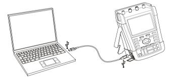
Figure 36. Connecting a Computer
