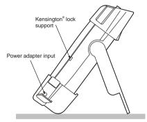
Figure 44. Using the Tilt Stand
