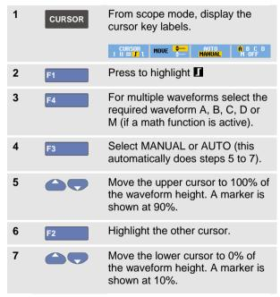
The reading shows the risetime from 10%-90% of the waveform amplitude.
