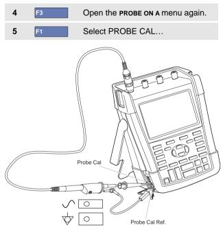
Figure 50. Adjusting Voltage Probes
