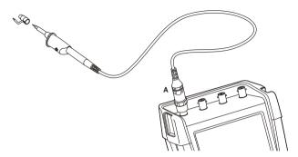
Figure 37. HF Voltage Probe Connection Using Ground Spring
