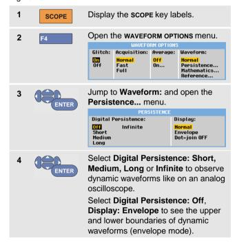
Select **Display: Dot-join: Off** to display measured samples only. Dot join off may be useful when measuring for example modulated signals or video signals.
