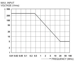
Figure 51. Max. Input Voltage vs. Frequency
