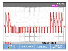
Figure 32. Measuring Interlaced Video Signals
