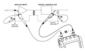
Figure 42. Correct connection of reference leads
