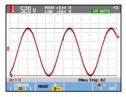
Figure 25. Voltage Measurement with Cursors
