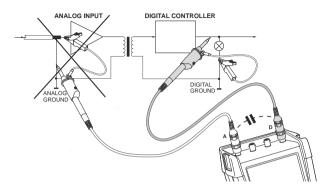
Figure 43. Wrong connection of reference leads
