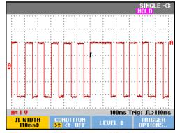
Figure 34. Triggering on Missing Pulses
