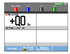
Figure 13. Making a Relative Measurement
