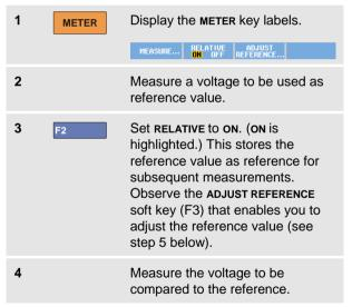
Now the large reading is the actual input value minus the stored reference value. The bargraph indicates the actual input value. The actual input value and the reference value are displayed below the large reading (ACTUAL: xxxx REFERENCE: xxx), see Figure 18.
