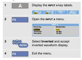
For example, a negative-going waveform is displayed as positive-going waveform which may provide a more meaningful view. An inverted display is identified by an inversed waveform identifier ( 1) at the right of the waveform, and in the status line below the waveform.
