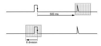
Figure 29. Trigger Delay or Pre-trigger View
