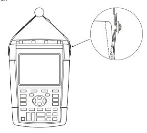
Figure 45. Fixing the Hangstrap
