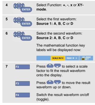
The sensitivity range of the mathematical result is equal to the sensitivity range of the least sensitive input divided by the scale factor.
