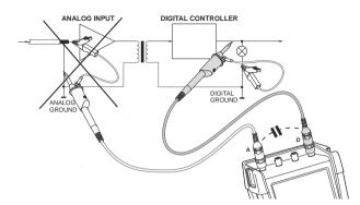
Figure 43. Wrong connection of reference leads
