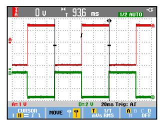
Figure 26. Time Measurement with Cursors
