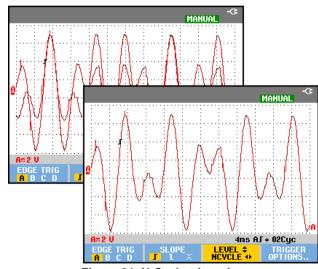
Figure 31. N-Cycle triggering
