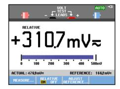
Figure 18. Making a Relative Measurement
