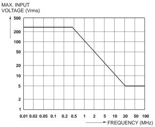
Figure 51. Max. Input Voltage vs. Frequency
