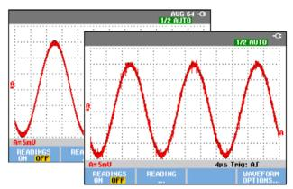
Figure 9. Smoothing a Waveform
