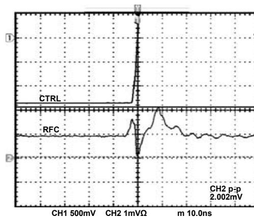
Figure 15. Video Feedthrough
