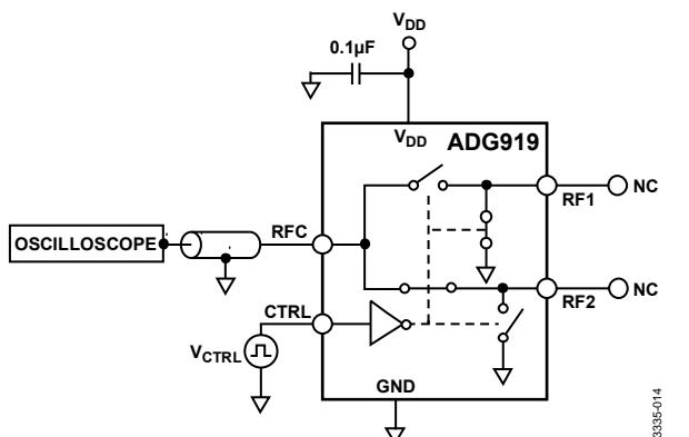
Figure 23. Video Feedthrough
