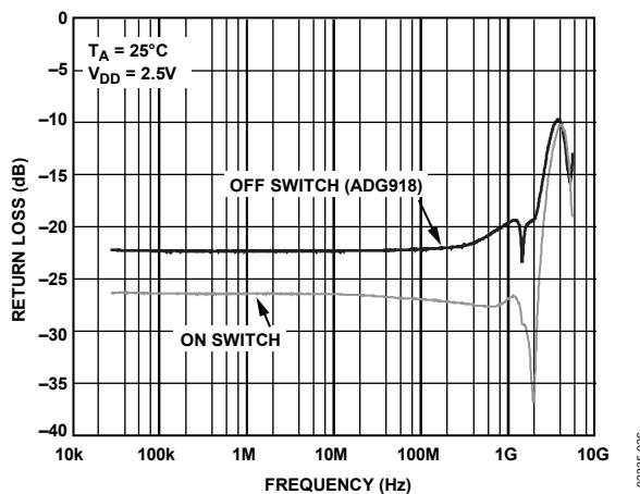
Figure 12. Return Loss vs. Frequency (RF1/RF2, S11)
