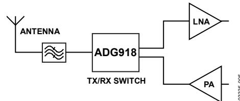
Figure 26. Wireless Metering
