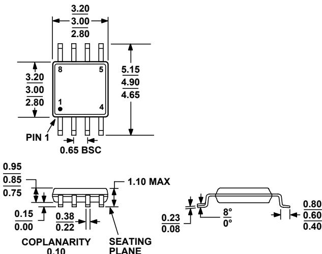
Figure 30. 8-Lead Mini Small Outline Package [MSOP]
