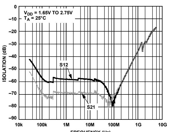
Figure 9. Isolation vs. Frequency over Supplies (RF1/RF2, ADG918)
