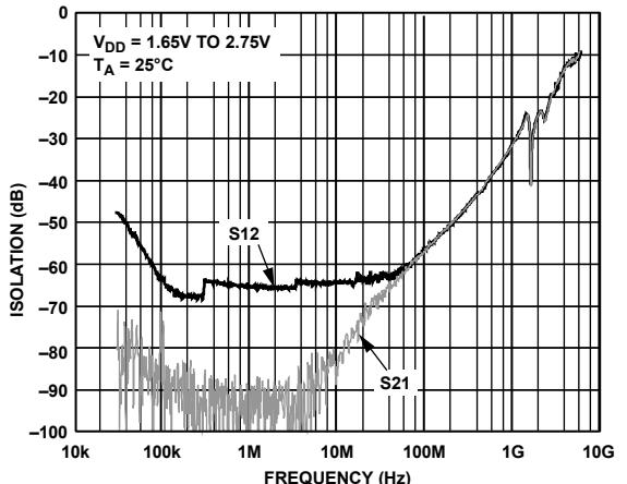
Figure 10. Isolation vs. Frequency over Supplies (RF1/RF2, ADG919)
