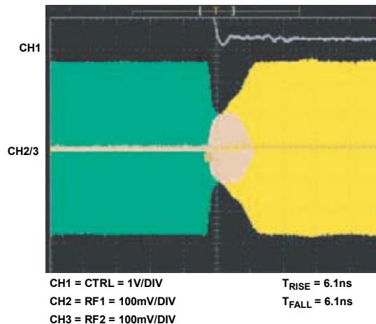
Figure 14. Switch Timing
