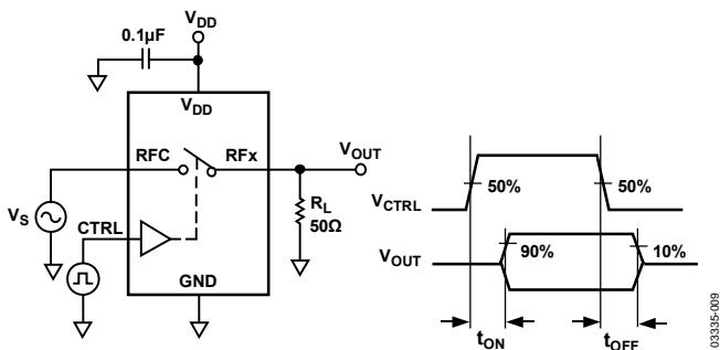
Figure 18. Switch Timing:  $t_{\text{ON}}, t_{\text{OFF}}$
