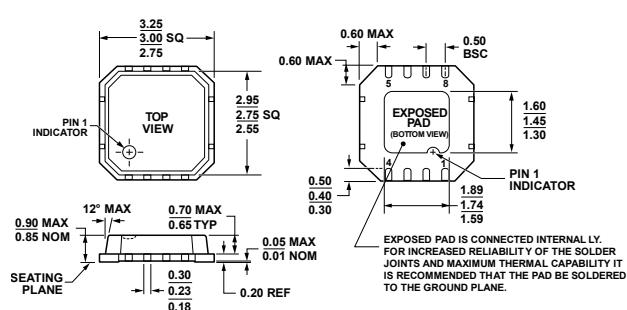
Figure 31. 8-Lead Lead Frame Chip Scale Package [LFCSP\_VD]
