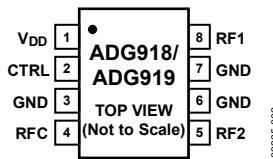
Figure 4. 8-Lead MSOP (RM-8) and
