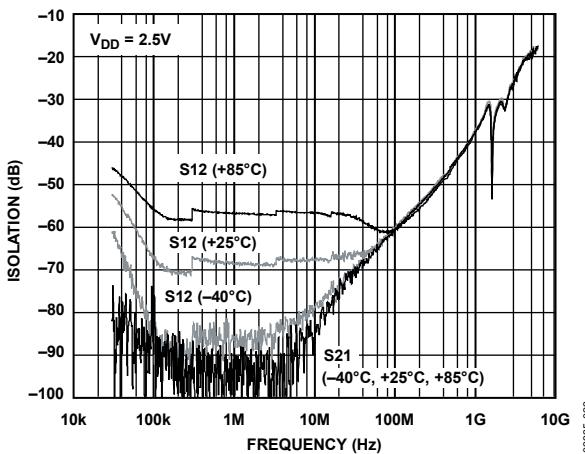
Figure 11. Isolation vs. Frequency over Temperature (RF1/RF2, ADG919)
