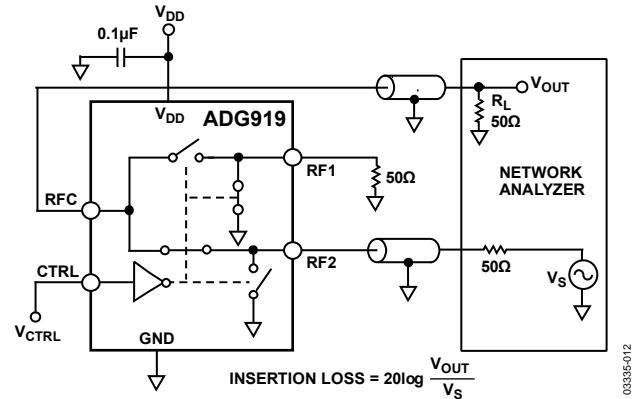
Figure 21. Insertion Loss
