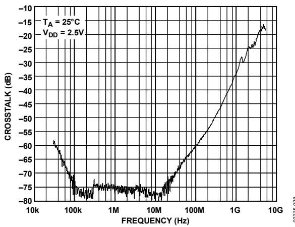
Figure 13. Crosstalk vs. Frequency (RF1/RF2, S12, S21)
