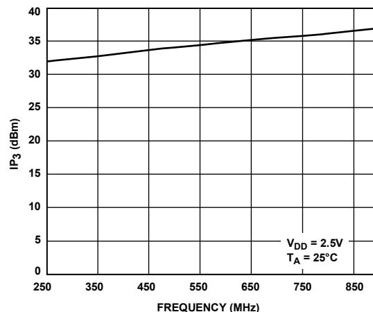
Figure 16. IP3 vs. Frequency
