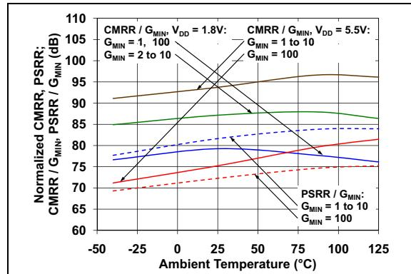
**FIGURE 2-16:** Normalized CMRR and PSRR vs. Ambient Temperature.
