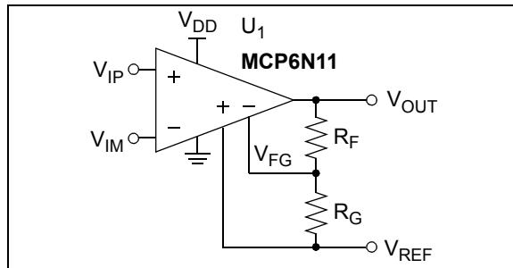
**FIGURE 4-1:** Standard Circuit.
