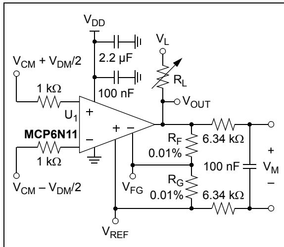
**FIGURE 1-7:** Test Circuit for Differential Mode.
