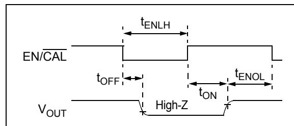
**FIGURE 1-5:**  $EN/\bar{CAL}$  Timing Diagram.
