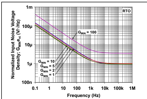
**FIGURE 2-38:** Normalized Input Noise Voltage Density vs. Frequency.
