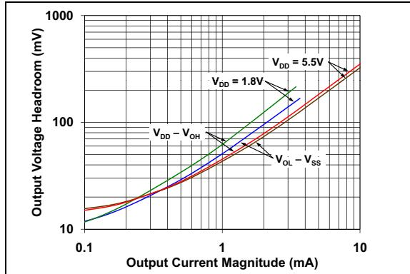
**FIGURE 2-27:** Output Voltage Headroom vs. Output Current.
