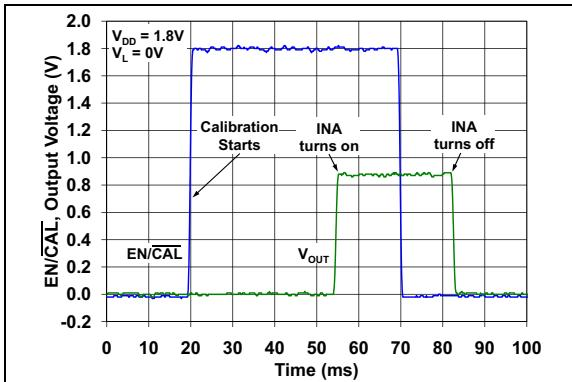
**FIGURE 2-52:**  $\text{EN}/\overline{\text{CAL}}$  and Output Voltage vs. Time, with  $V_{DD} = 1.8\text{V}$ .
