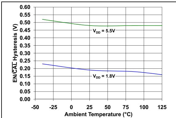
**FIGURE 2-54:**  $\text{EN}/\overline{\text{CAL}}$  Hysteresis vs. Ambient Temperature.
