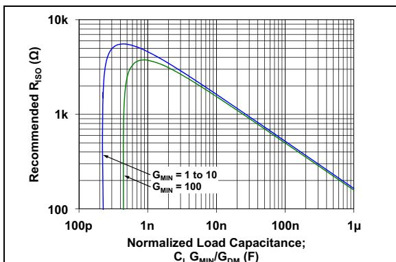
**FIGURE 4-9:** Recommended  $R_{ISO}$  Values for Capacitive Loads.
