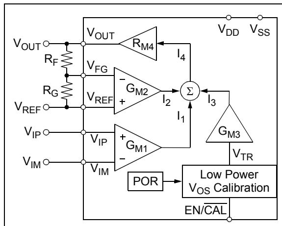
**FIGURE 4-2:** MCP6N11 Block Diagram.
