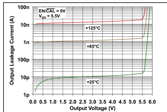
**FIGURE 2-59:** Output Leakage Current vs. Output Voltage.
