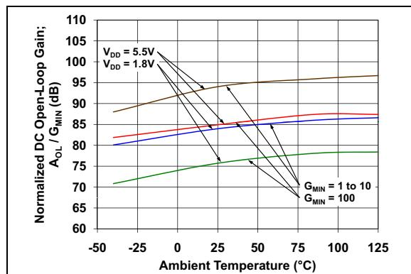
**FIGURE 2-17:** Normalized DC Open-Loop Gain vs. Ambient Temperature.
