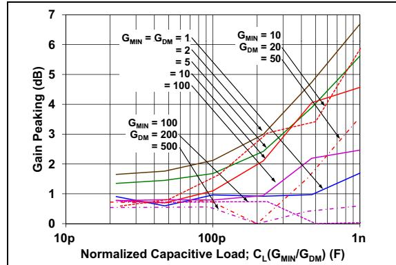
**FIGURE 2-37:** Gain Peaking vs. Normalized Capacitive Load.
