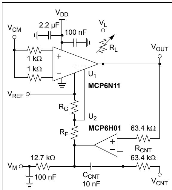
**FIGURE 1-6:** Test Circuit for Common Mode (Input Offset).
