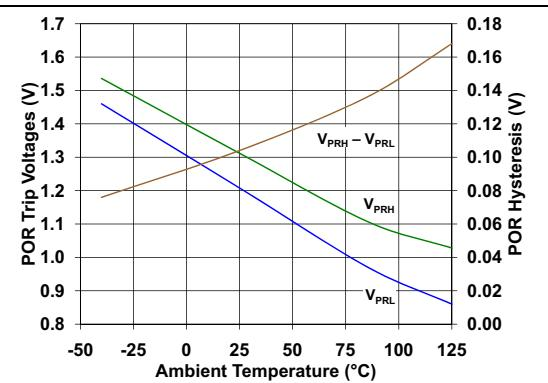
**FIGURE 2-57:** POR Trip Voltages and Hysteresis vs. Temperature.
