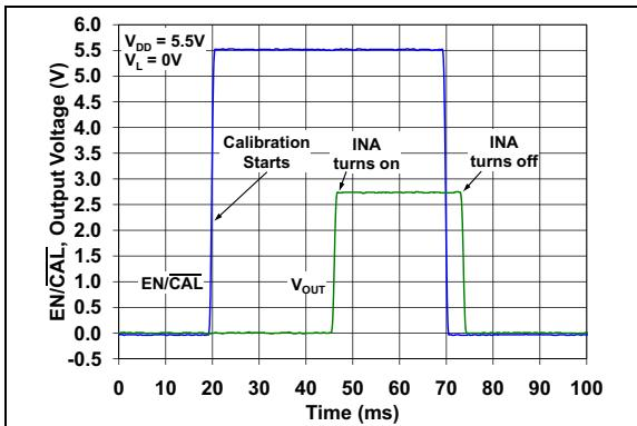
**FIGURE 2-53:**  $\text{EN}/\overline{\text{CAL}}$  and Output Voltage vs. Time, with  $V_{DD} = 5.5\text{V}$
