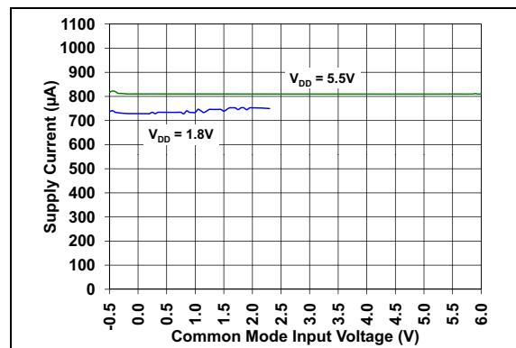
**FIGURE 2-31:** Supply Current vs. Common Mode Input Voltage.
