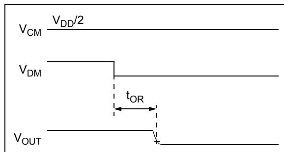
**FIGURE 1-3:** Output Overdrive Recovery Timing Diagram.
