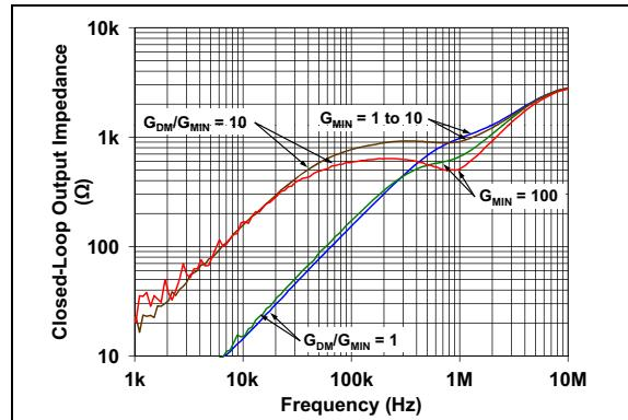
**FIGURE 2-36:** Closed-Loop Output Impedance vs. Frequency.
