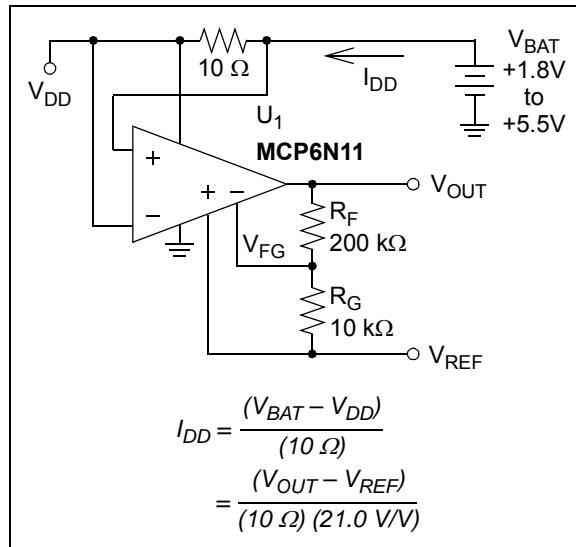
**FIGURE 4-13:** High Side Current Detector.
