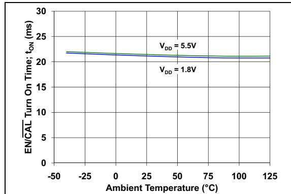
**FIGURE 2-55:**  $\text{EN}/\overline{\text{CAL}}$  Turn On Time vs. Ambient Temperature.
