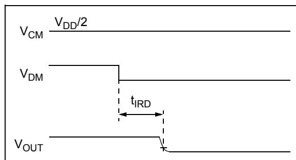
**FIGURE 1-2:** Differential Mode Input Overdrive Recovery Timing Diagram.
