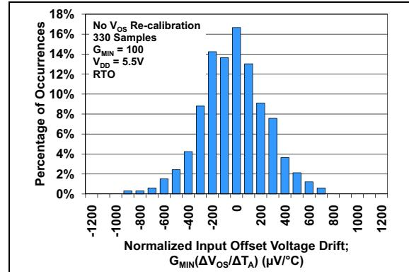
**FIGURE 2-4:** Normalized Input Offset Voltage Drift, with  $G_{MIN} = 100$ .
