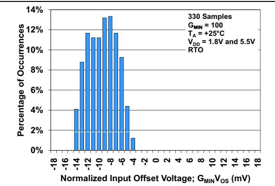
**FIGURE 2-2:** Normalized Input Offset Voltage, with  $G_{MIN} = 100$ .
