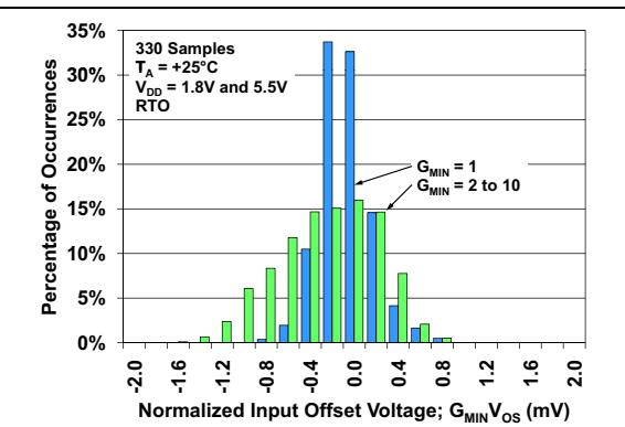
**FIGURE 2-1:** Normalized Input Offset Voltage, with  $G_{MIN} = 1$  to 10.
