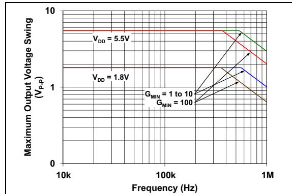
**FIGURE 2-46:** Maximum Output Voltage Swing vs. Frequency.
