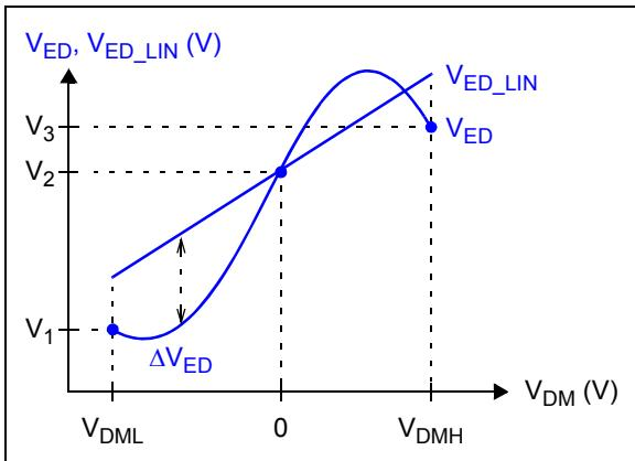
**FIGURE 1-9:** Differential Input Error vs. Differential Input Voltage.
