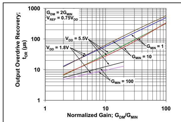
**FIGURE 2-49:** Output Overdrive Recovery Time vs. Normalized Gain.
