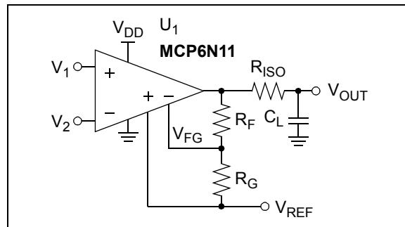
**FIGURE 4-8:** Output Resistor,  $R_{ISO}$  stabilizes large capacitive loads.
