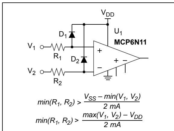
**FIGURE 4-6:** Protecting the Analog Inputs Against High Currents.
