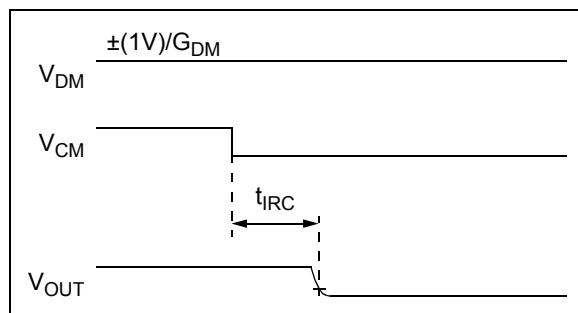
**FIGURE 1-1:** Common Mode Input Overdrive Recovery Timing Diagram.
