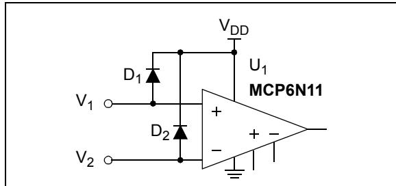
**FIGURE 4-5:** Protecting the Analog Inputs Against High Voltages.
