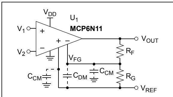
**FIGURE 4-10:** Simple Gain Circuit with Parasitic Capacitances.
