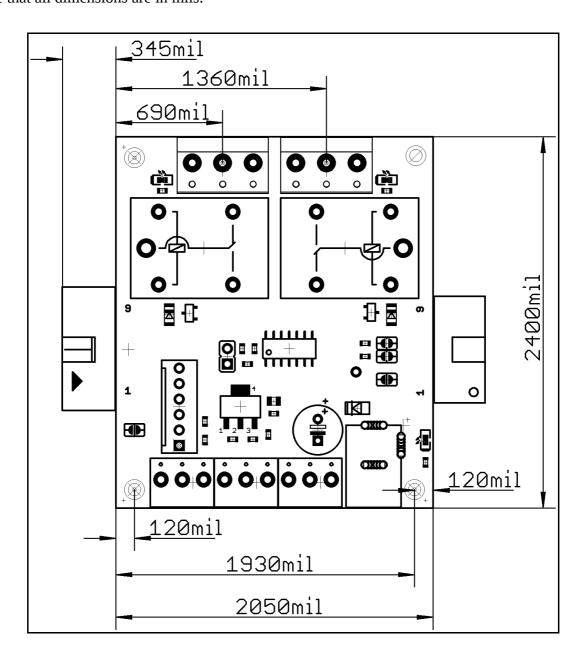
The three highest elements on the board in order from the tallest to the shortest are: relay T1 - 0.600" (15.25 mm) over the pcb; relay T2 - 0.600" (15.25 mm); ICSP connector -0.450" (11.43 mm).
