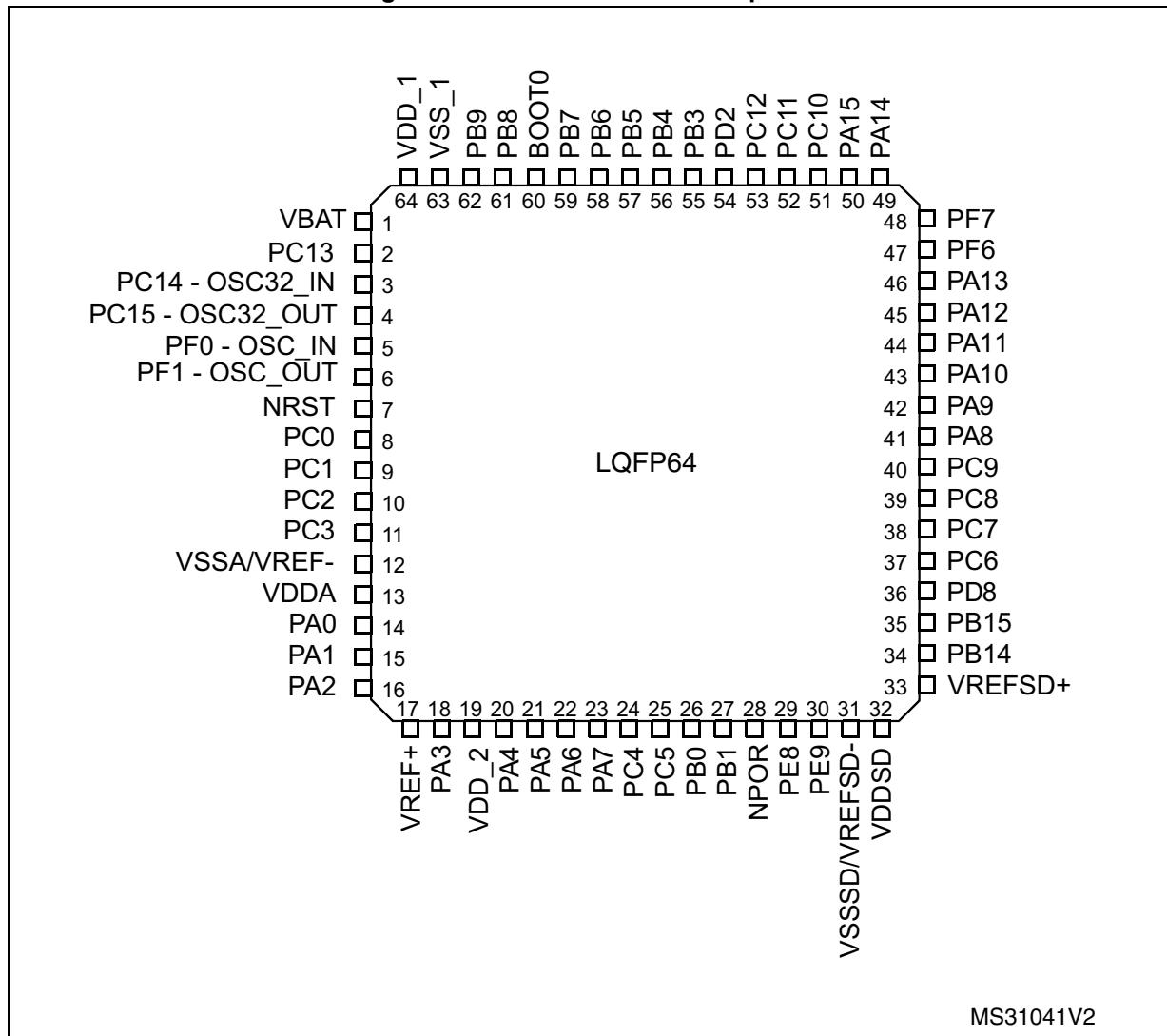
1. The above figure shows the package top view.
