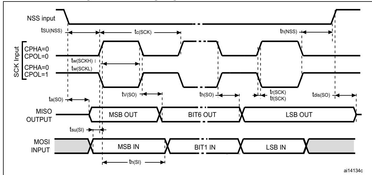
Figure 24. SPI timing diagram - slave mode and CPHA = 1<sup>(1)</sup>
