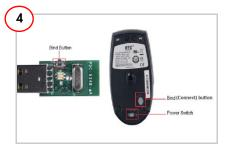
Turn on the mouse. Press the bind button on the bridge; the red LED blinks. Press the bind button on the mouse to bind it with the bridge.
