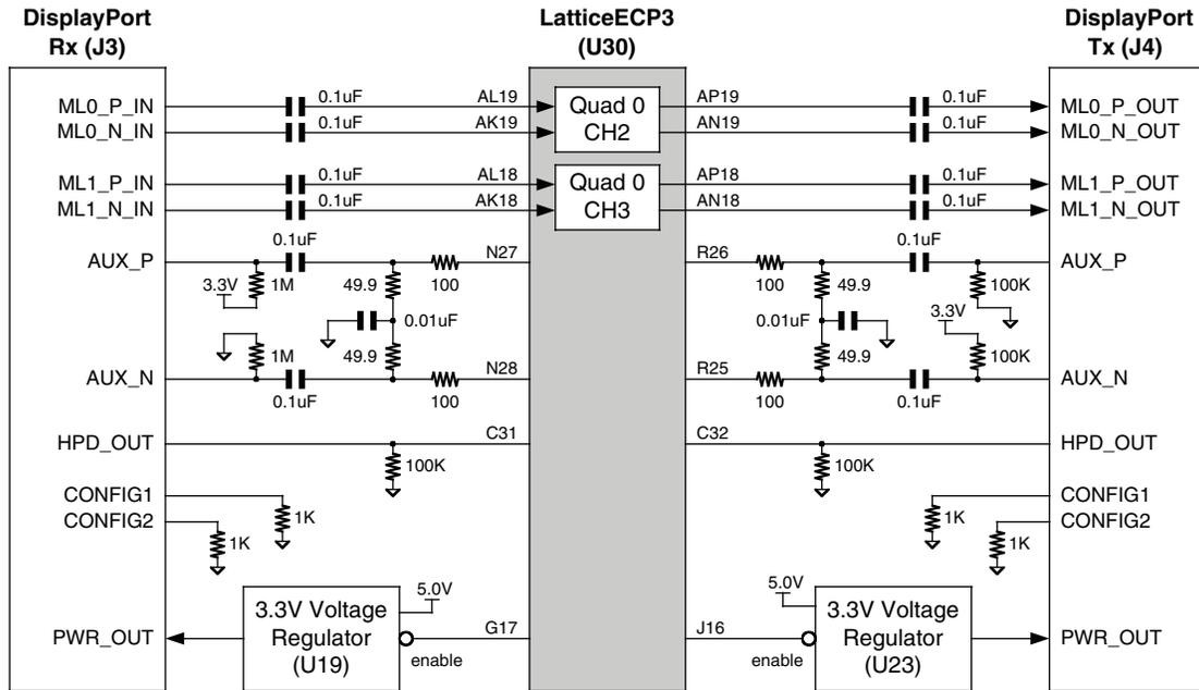
Table 17 shows the pin connections of the DisplayPort video interface.
