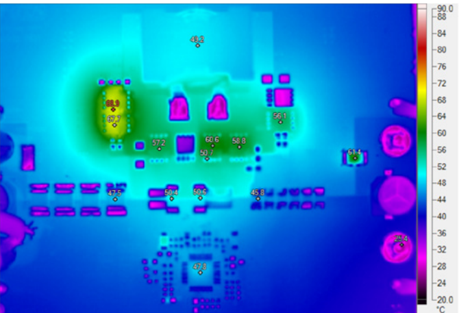
Figure 8. DC2519A Thermal Performance at 48V IN , 48V OUT , 10A Load Current with No Forced Airflow
