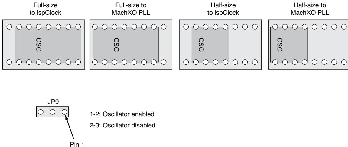
*Note: XU2 pin 9 is routed to one of the two PLLs included on larger MachXO devices. These MachXO PLLs are not available on the MachXO640 device. XU2 pin 9 provides input to the PLL\_T input pin M5.*
