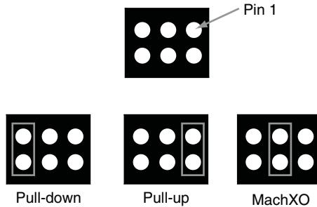
JP11 - JP17 configure all of the ispClock features. Table 11 shows which jumper block controls which ispClock pin. Refer to the ispClock5610 Family Data Sheet to understand what function each pin performs.
