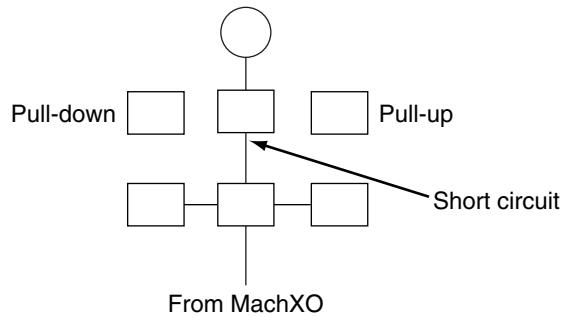
The resistor pads are 0603 surface mount form factor. The 0603 resistor in the center has a short-circuit trace between the resistor pads. This permits the signal to be driven to the prototype area without the addition of a SMT zero ohm resistor. If a series resistor with a non-zero value is needed, this short-circuit trace can be removed.
