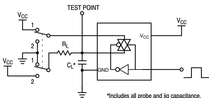
**Figure 6. Propagation Delay Output Enable/Disable Test Set-Up**
