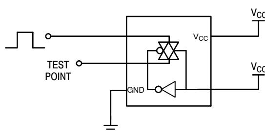
**Figure 5. Propagation Delay Test Set-Up**
