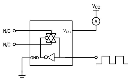
**Figure 7. Power Dissipation Capacitance Test Set-Up**
