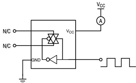
Figure 7. Power Dissipation Capacitance Test Set-Up
