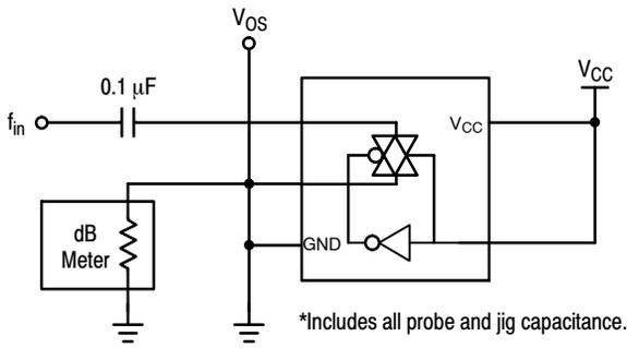
**Figure 8. Maximum On-Channel Bandwidth Test Set-Up**
