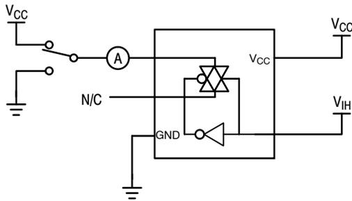
Figure 4. Maximum On-Channel Leakage Current Test Set-Up
