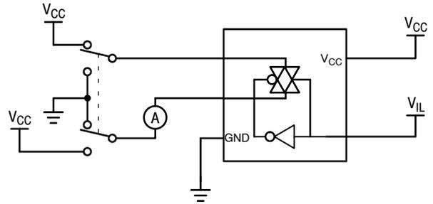
Figure 3. Maximum Off-Channel Leakage Current Test Set-Up
