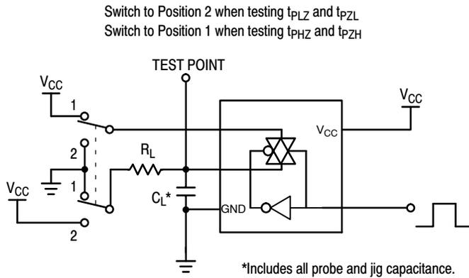
Figure 6. Propagation Delay Output Enable/Disable Test Set-Up
