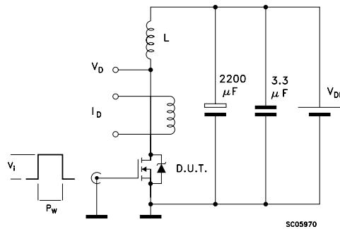
**Figure 16. Unclamped inductive waveform**
