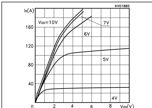
Figure 4. Transfer characteristics
