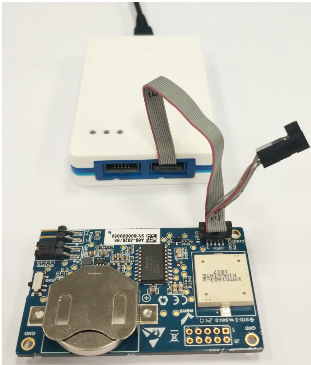
Figure 4-1. Connection of the Board and Programmer
