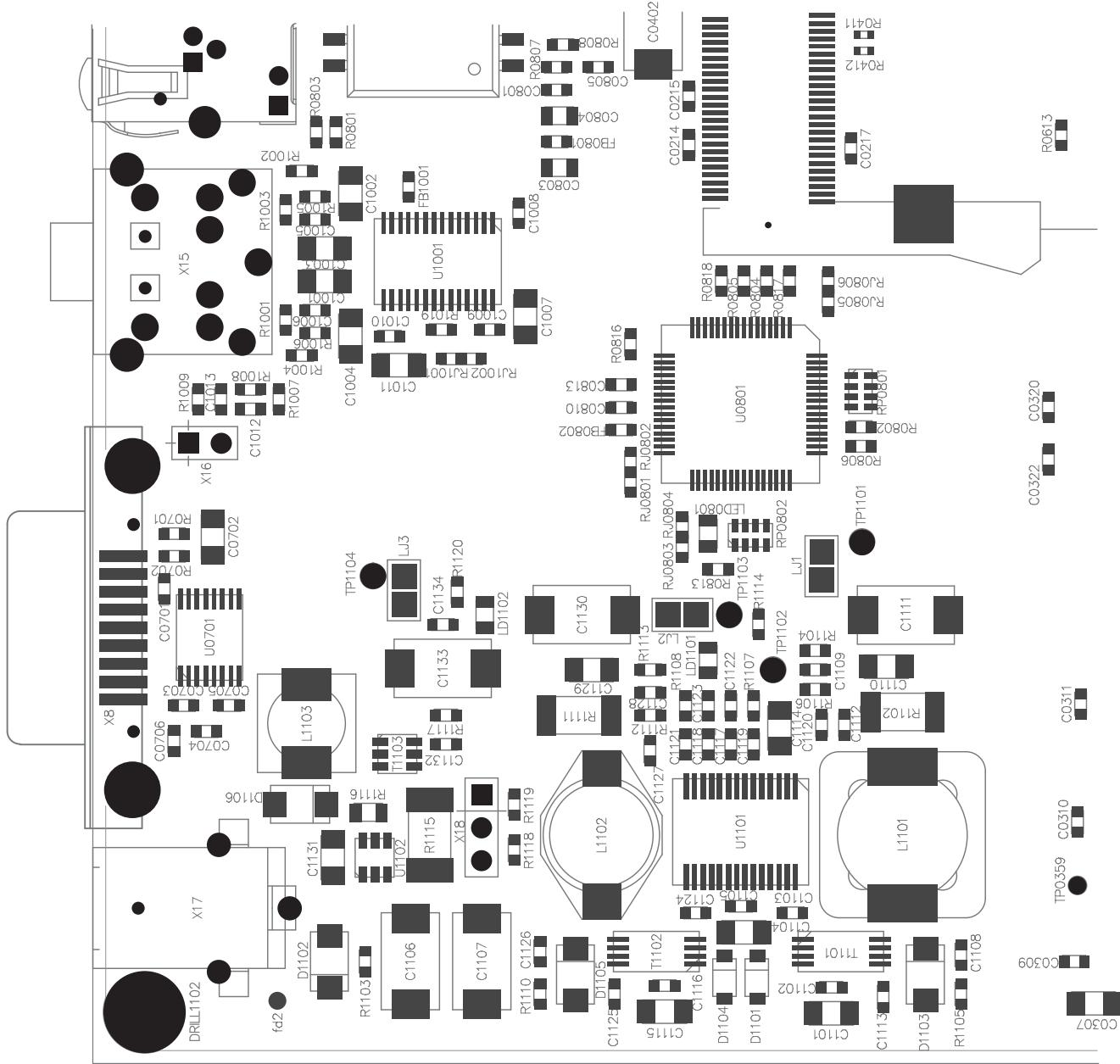
**Figure 26. Assembly Diagram, Section 4 Detail**
