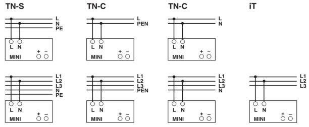
The 100 V AC ... 240 V AC connection is made using the L and N screw connections.
