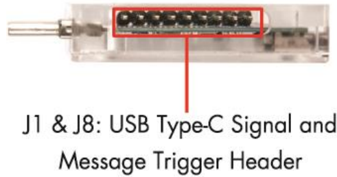
Figure 3-4: CY4500 EZ-PD™ Protocol Analyzer Board (Side View)
