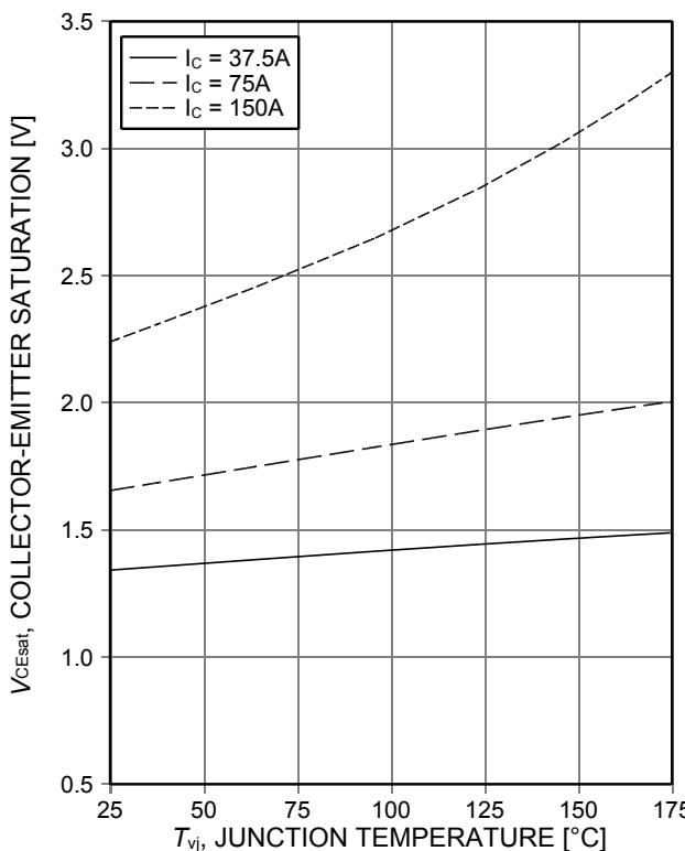
Figure 7. Typical collector-emitter saturation voltage as
