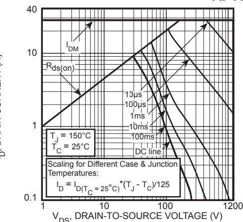
Figure 10, Maximum Forward Safe Operating Area
