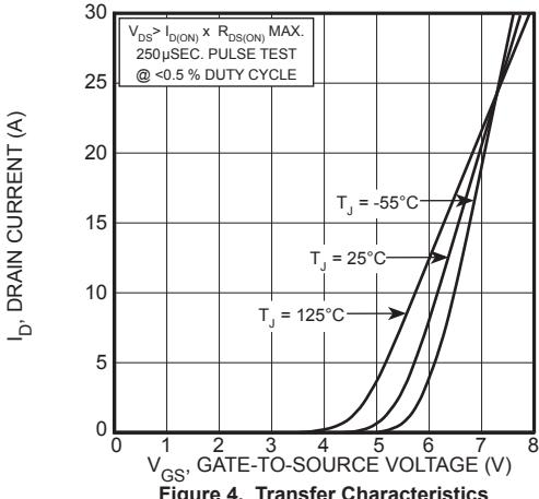
Figure 4, Transfer Characteristics
