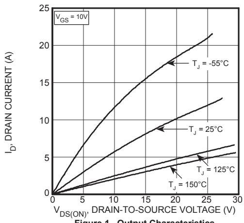
Figure 1, Output Characteristics
