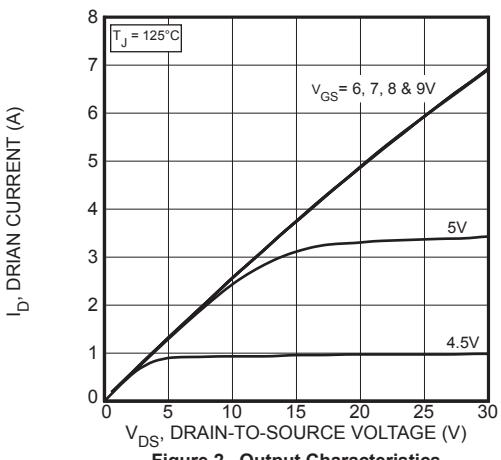
Figure 2, Output Characteristics
