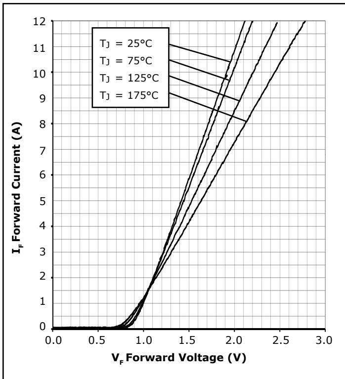
Figure 1. Forward Characteristics
