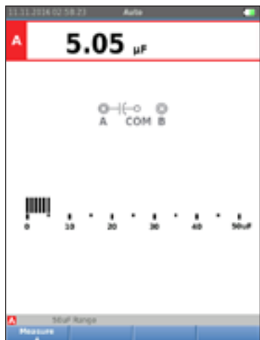
A single test tool measures volts, ohms, amps or capacitance, in addition to displaying waveforms.
