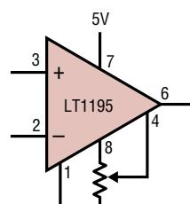
INPUT OFFSET VOLTAGE CAN BE ADJUSTED OVER A  $\pm 150mV$  RANGE WITH A 1k to 10k POTENTIOMETER.
