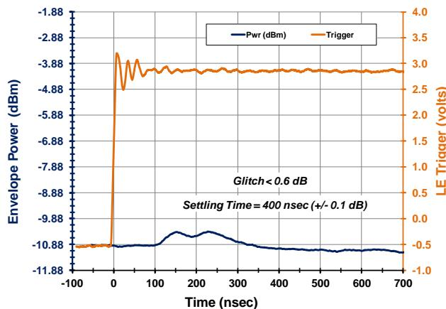
The graphs above show the transient overshoot and settling time performance for both the MSB+ and MSB- cases for the F1950. The device settles very quickly (~400) nsec with benign (~0.5) dB overshoot.
