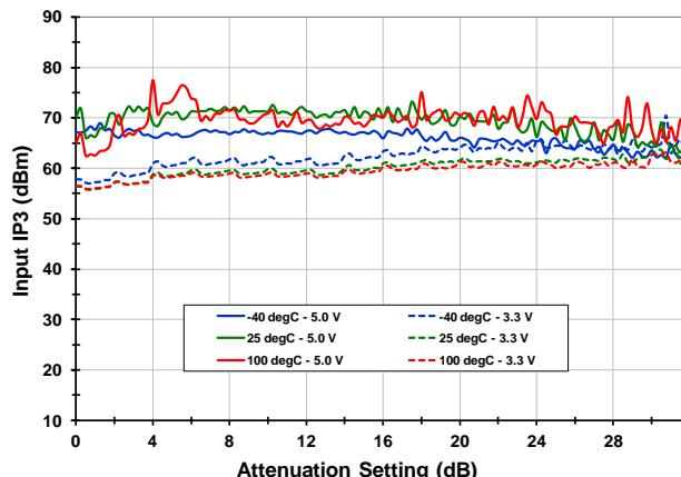
**Input IP3 [ $f_{RF} = 1900$  MHz]**
