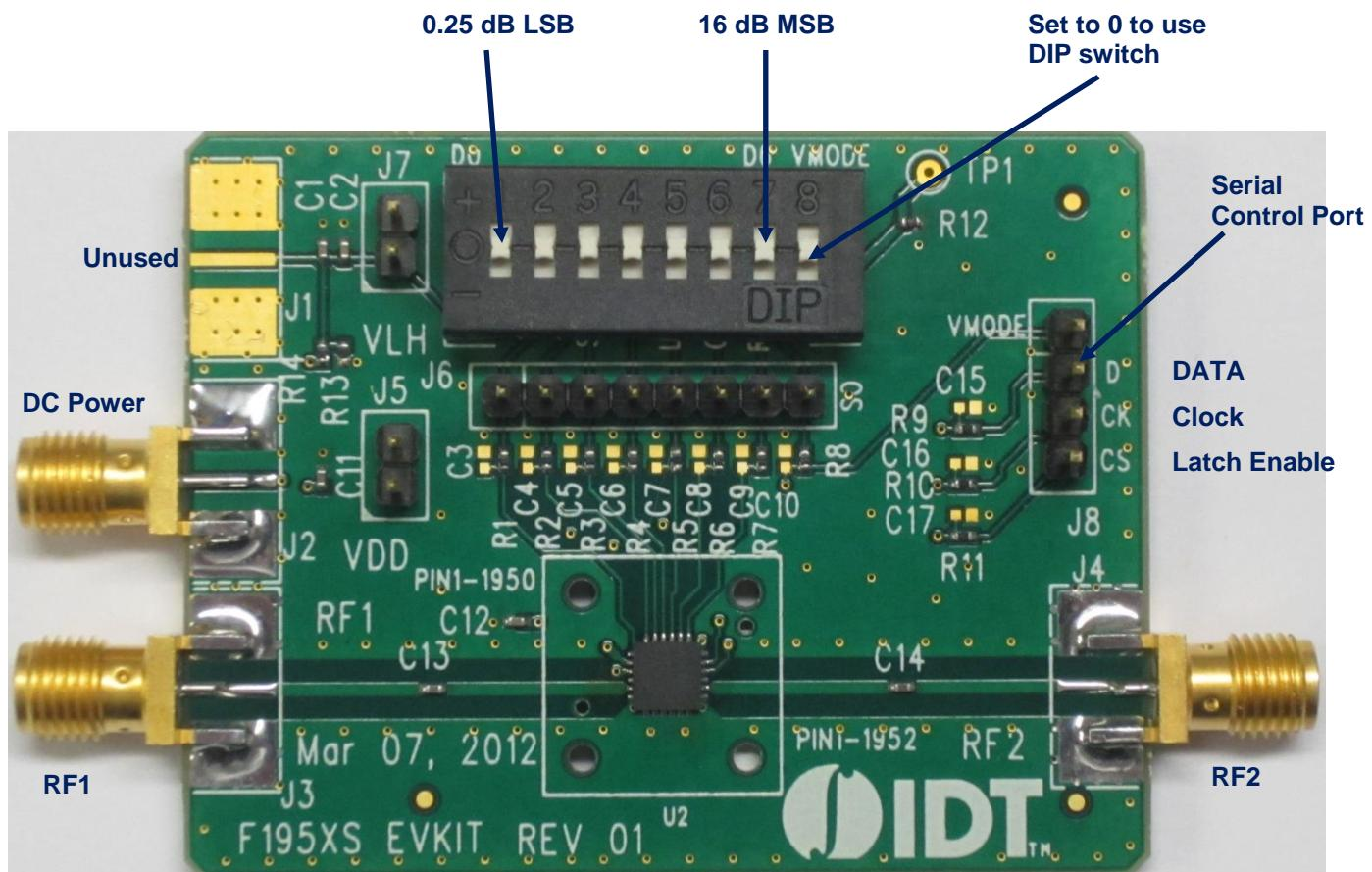
**7-bit 0.25 dB Digital Step Attenuator**
