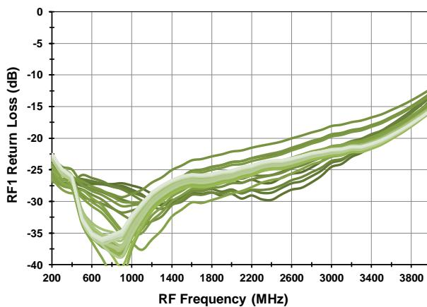
**S<sub>22</sub> vs. Frequency [T<sub>CASE</sub> = +25C, 0.75 dB steps]**
