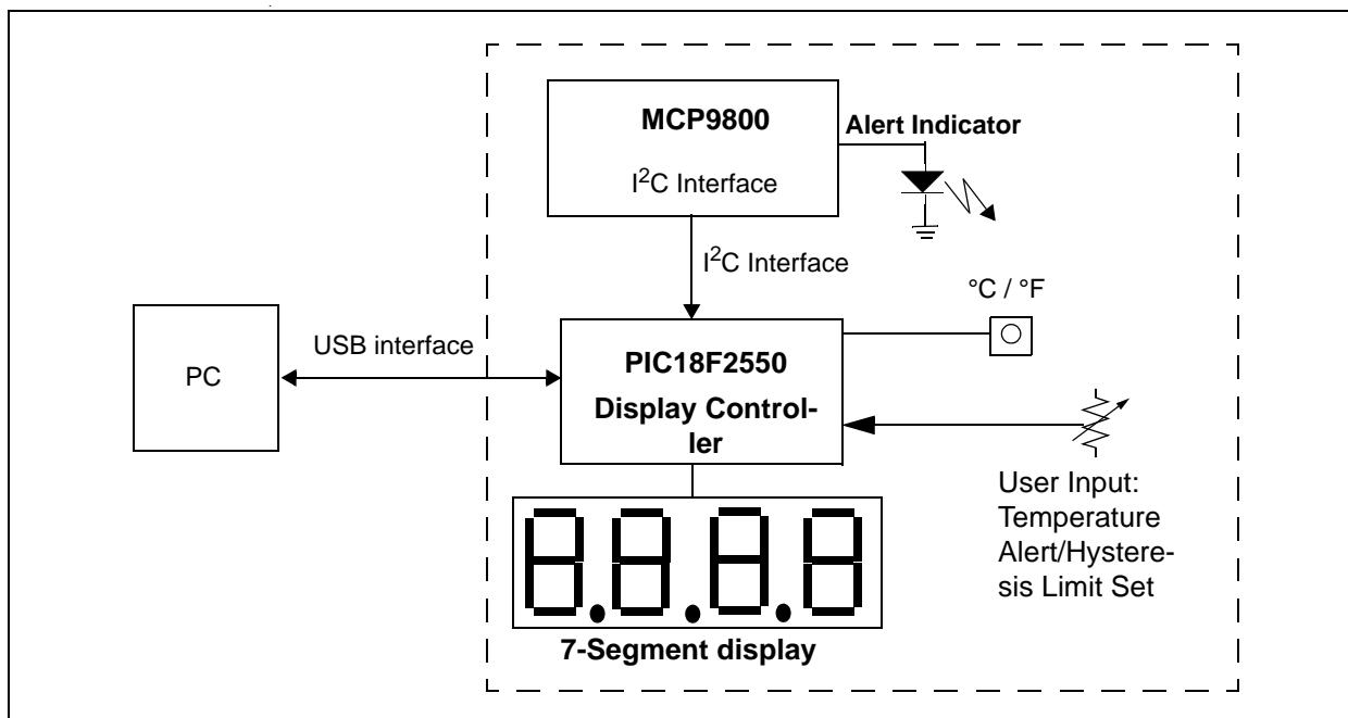
**FIGURE 2-1:** MCP9800 Temperature Sensor Demo Board Block Diagram.
