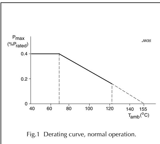
Fig.1 Derating curve, normal operation.
