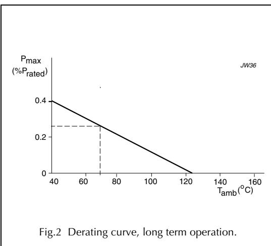
Fig.2 Derating curve, long term operation.
