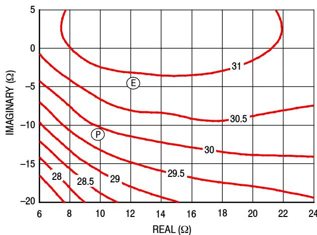
Figure 16. P3dB Load Pull Gain Contours (dB)
