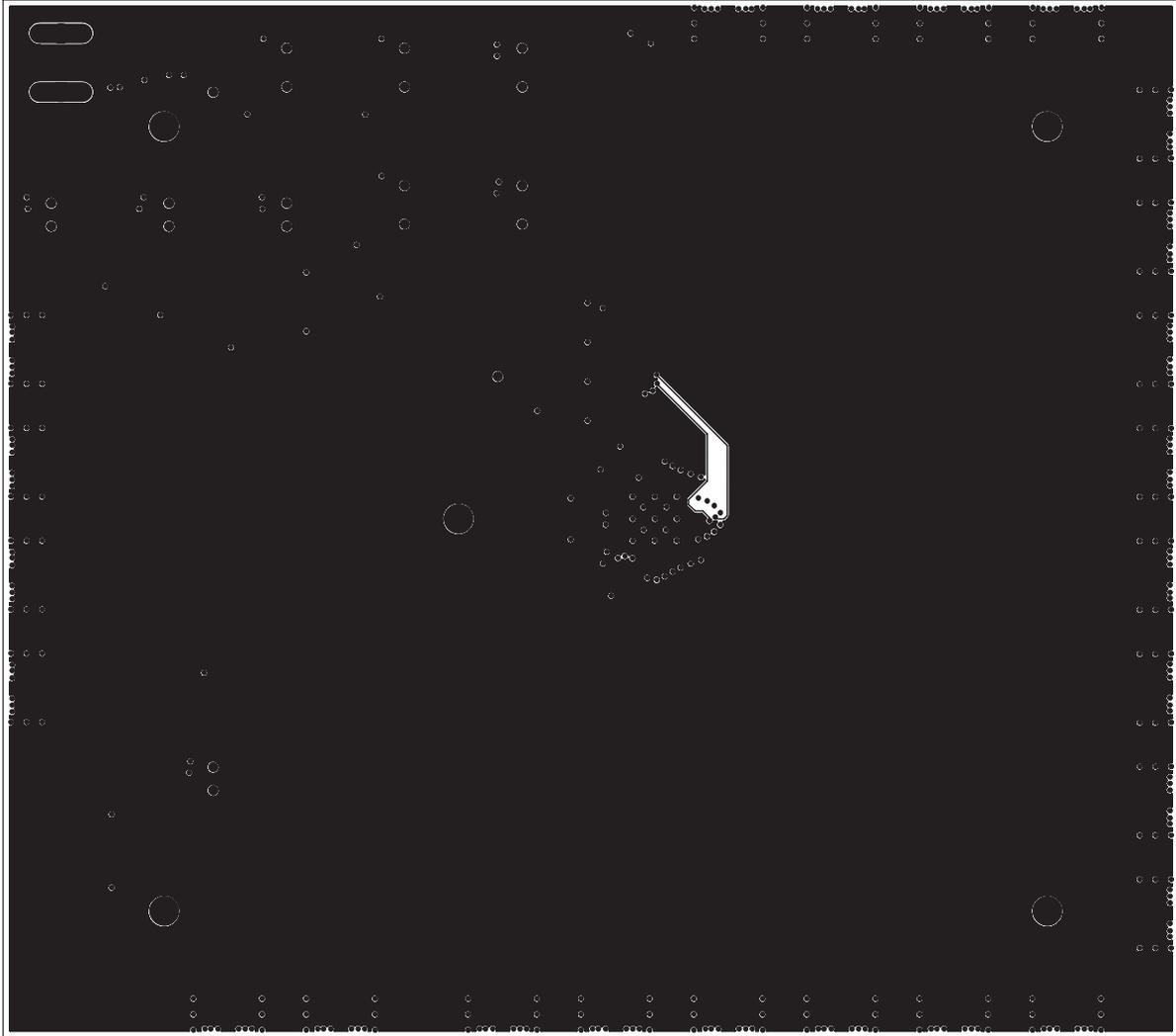
Figure 5. MAX3678 EV Kit PCB Layout—Power Plane
