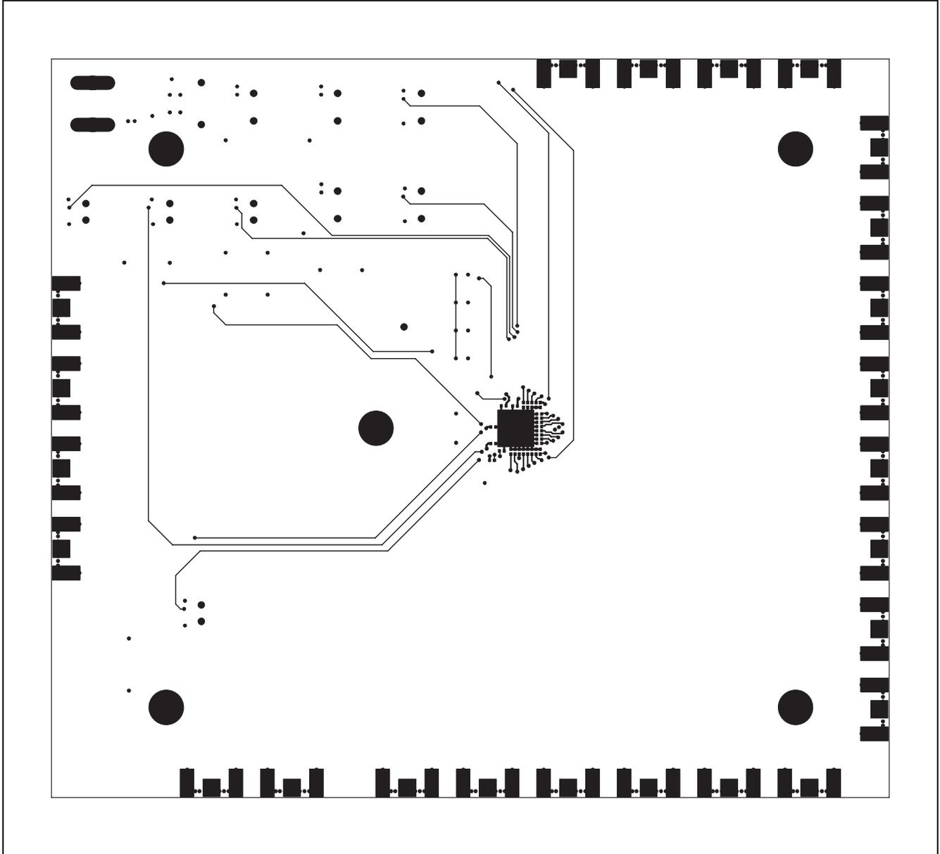
Figure 6. MAX3678 EV Kit PCB Layout—Solder Side
