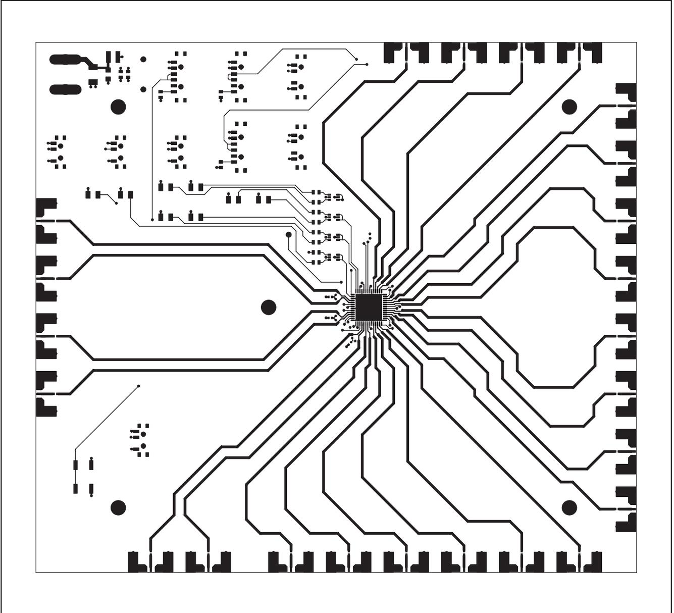
Figure 3. MAX3678 EV Kit PCB Layout—Component Side
