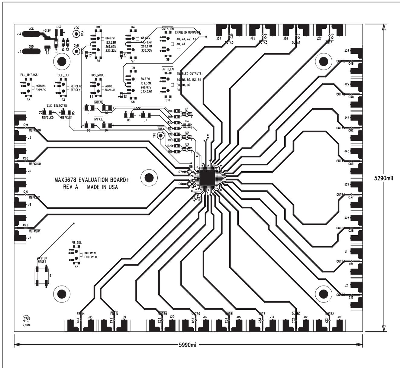
Figure 2. MAX3678 EV Kit Component Placement Guide—Component Side
