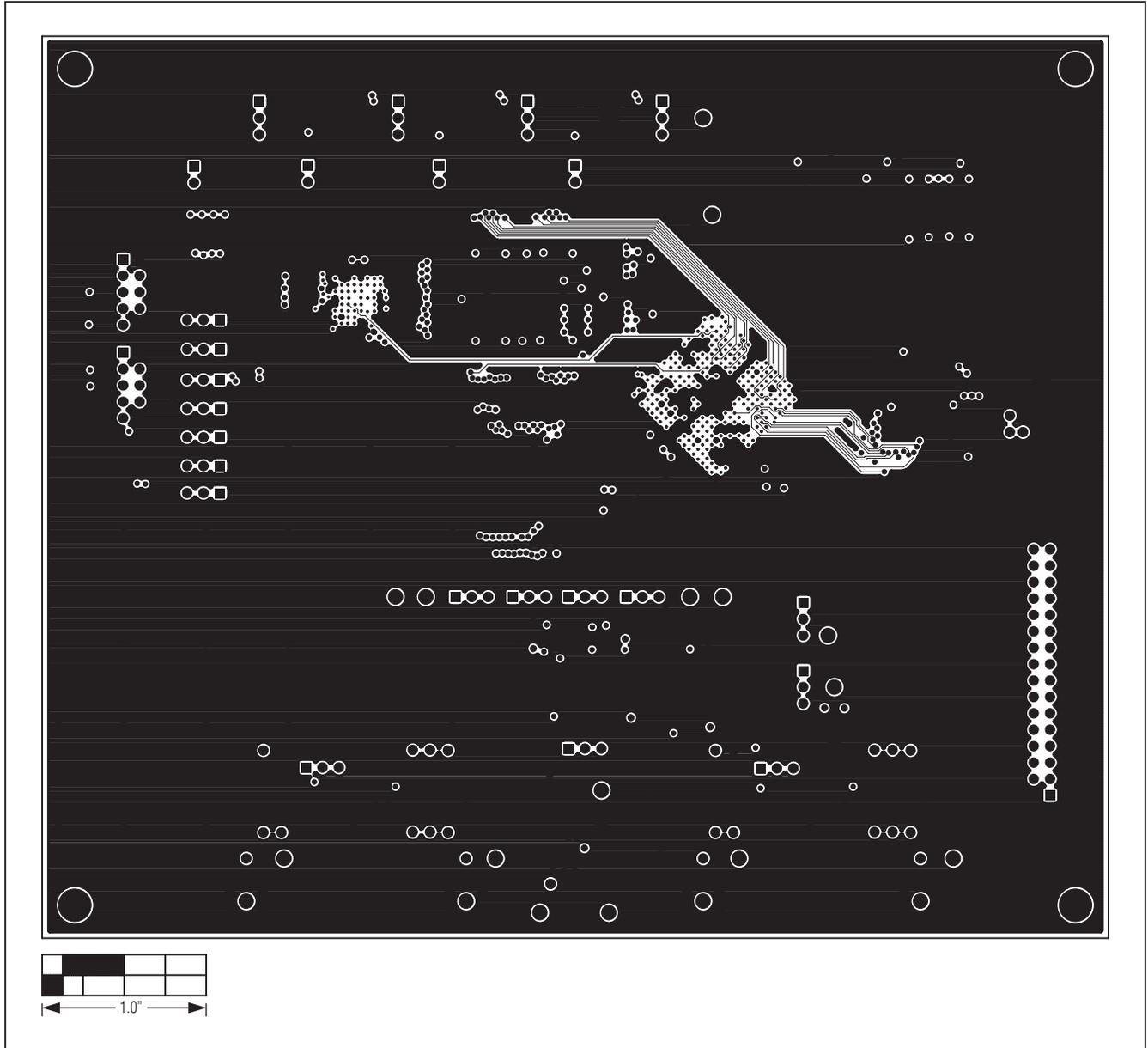
Figure 14. MAX11666 EV Kit PCB Layout—Layer 7
