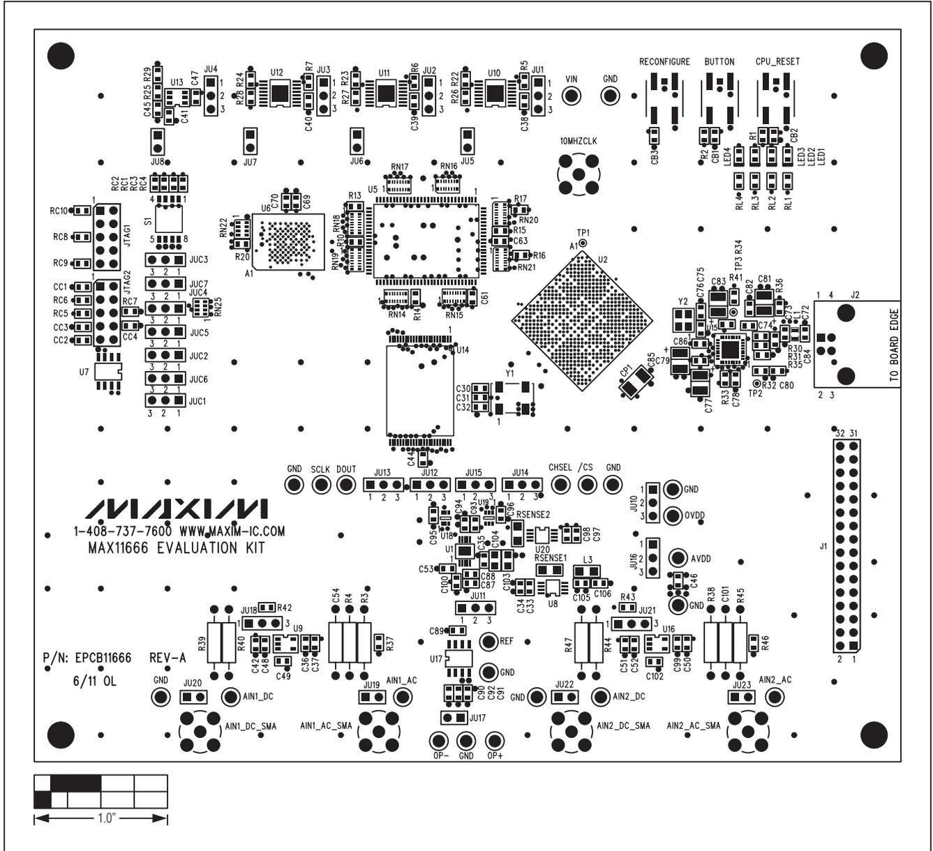
Figure 7. MAX11666 EV Kit Component Placement Guide—Top
