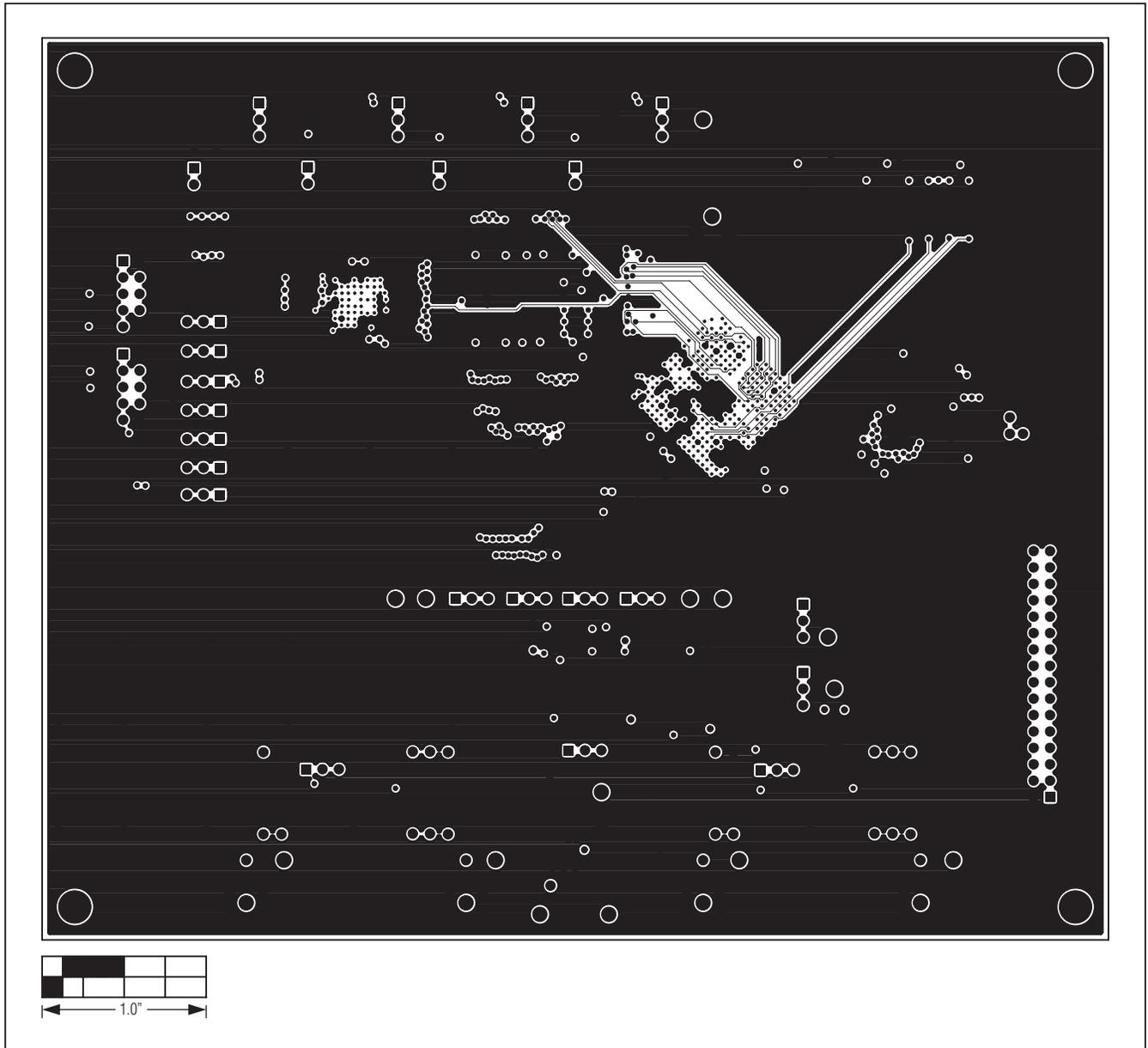
Figure 11. MAX11666 EV Kit PCB Layout—Layer 4
