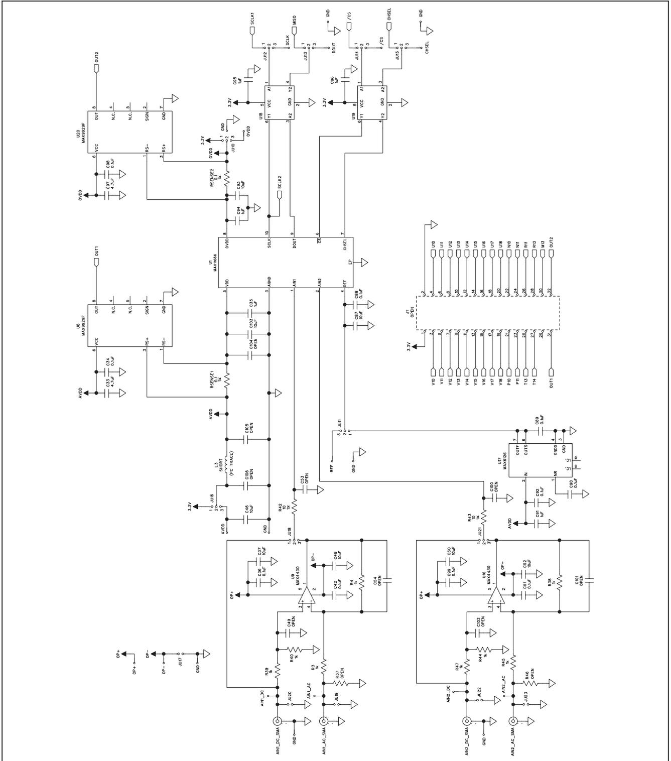
Figure 6a. MAX11666 EV Kit Schematic (Sheet 1 of 12)
