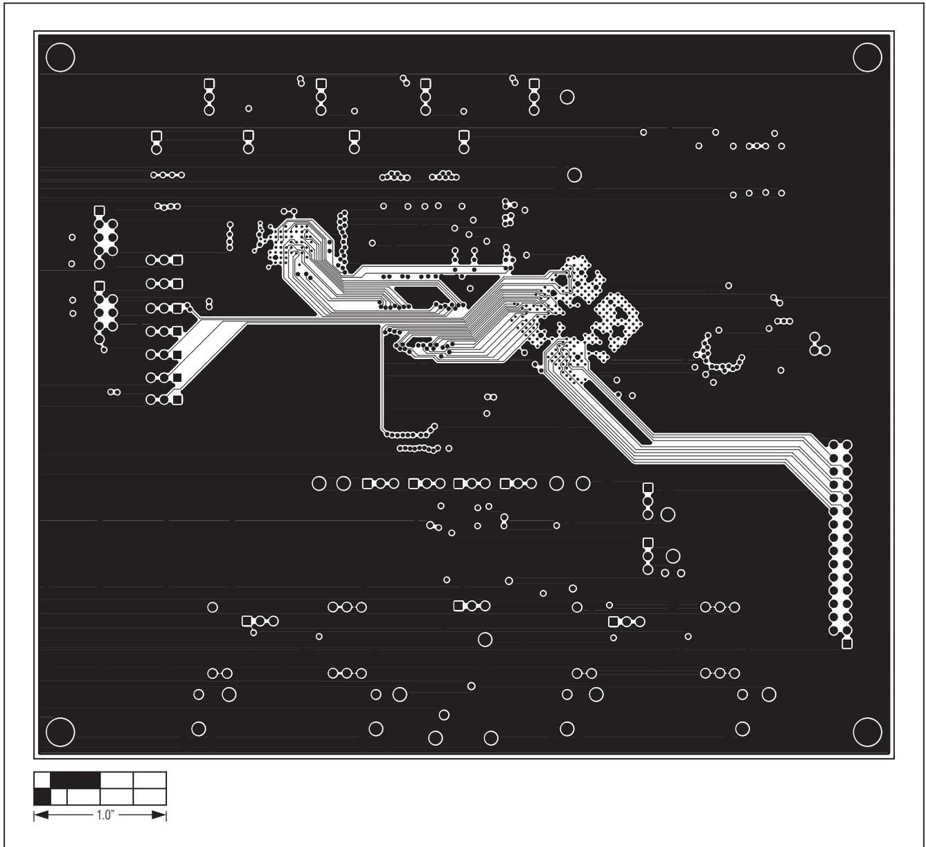
Figure 17. MAX11666 EV Kit PCB Layout—Layer 10
