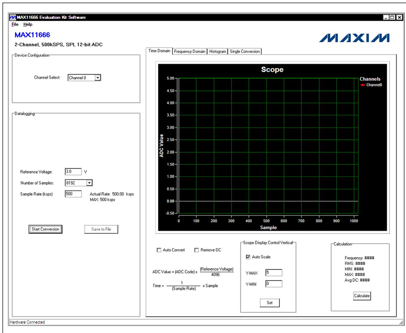
Figure 1. MAX11666 EV Kit Software Main Window
