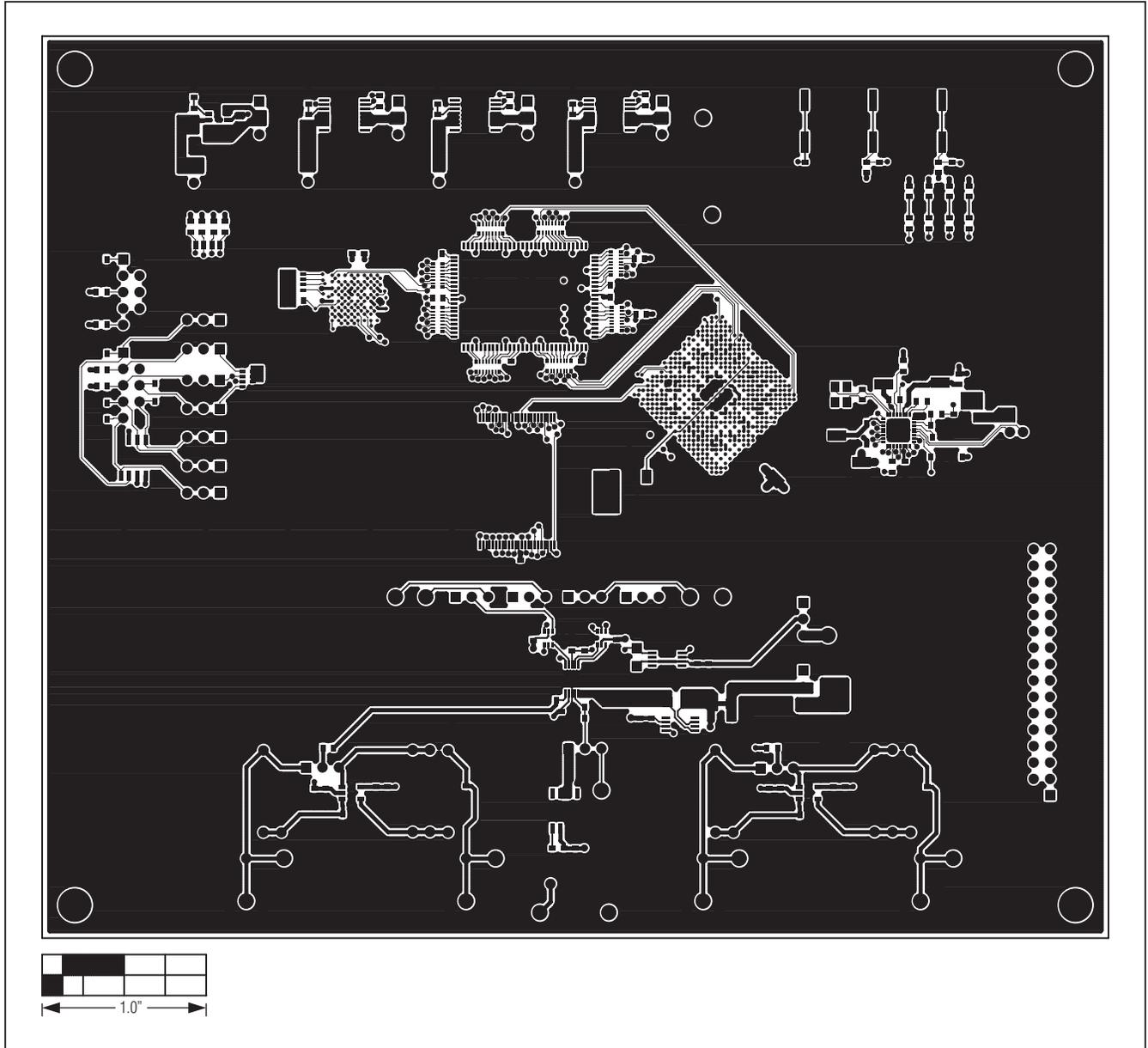
Figure 8. MAX11666 EV Kit PCB Layout—Component Side
