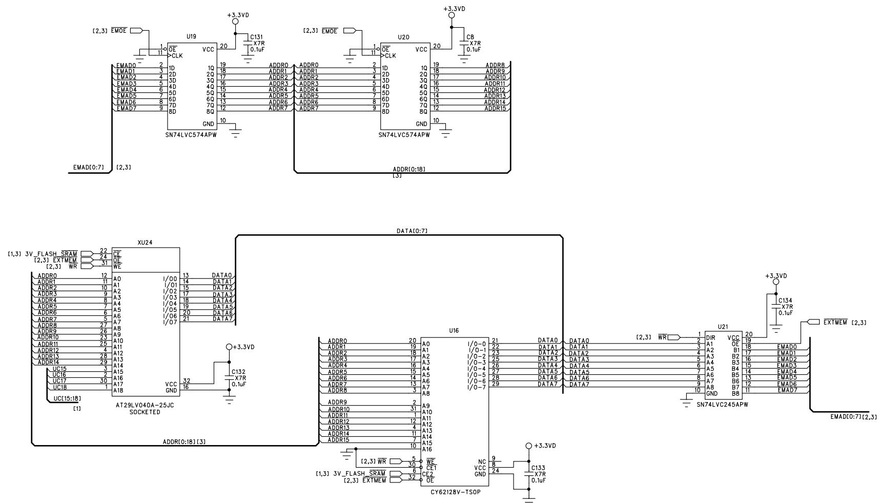
**SRAM\_FLASH** is used to select FLASH or SRAM.
