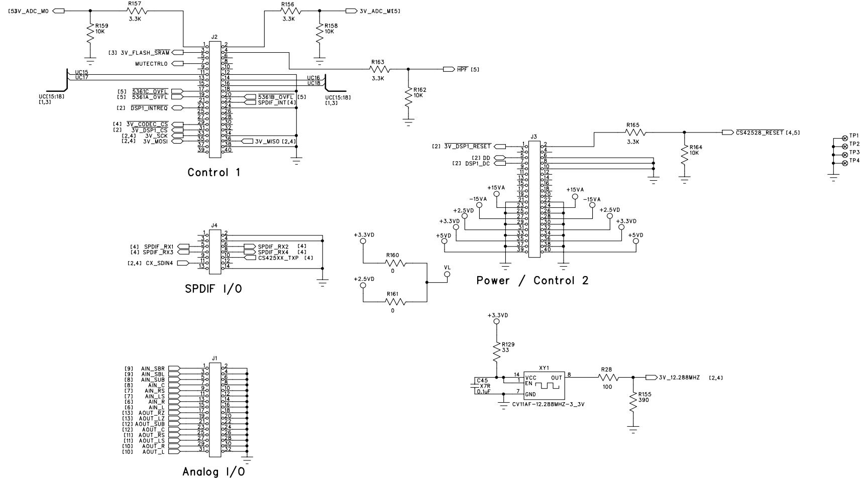
Connectors line up with UDSP interface, and should be mounted on the bottom of the board.
