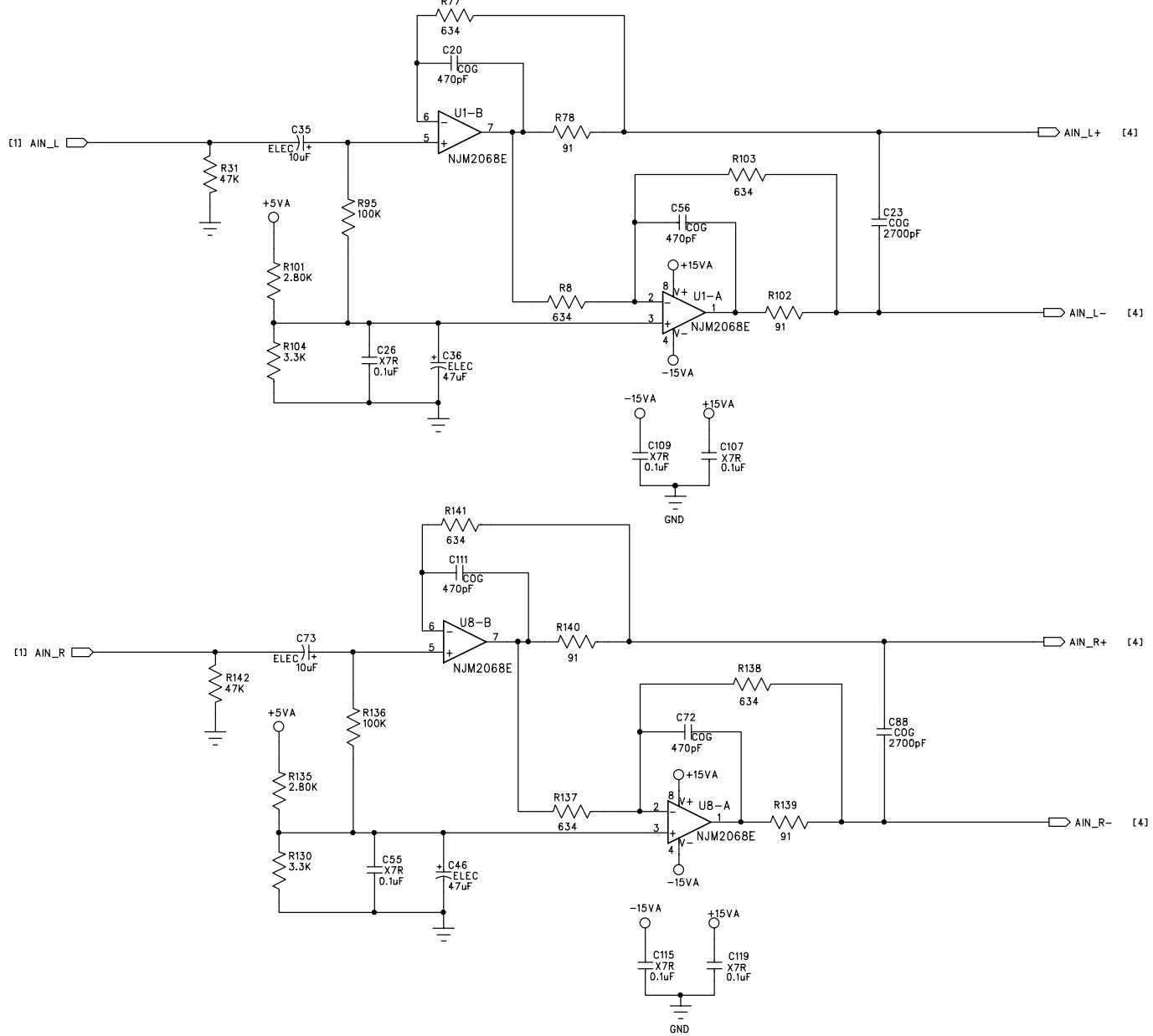
**Figure 11. L/R Input Filters**
