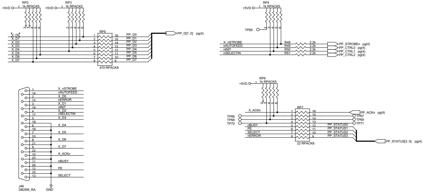
**Figure 27. UDSP - Parallel Port Interface**
