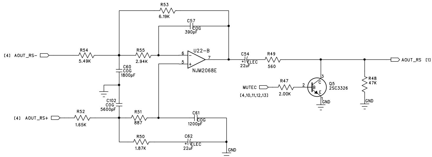
**Figure 16. Ls/Rs Output Filters**
