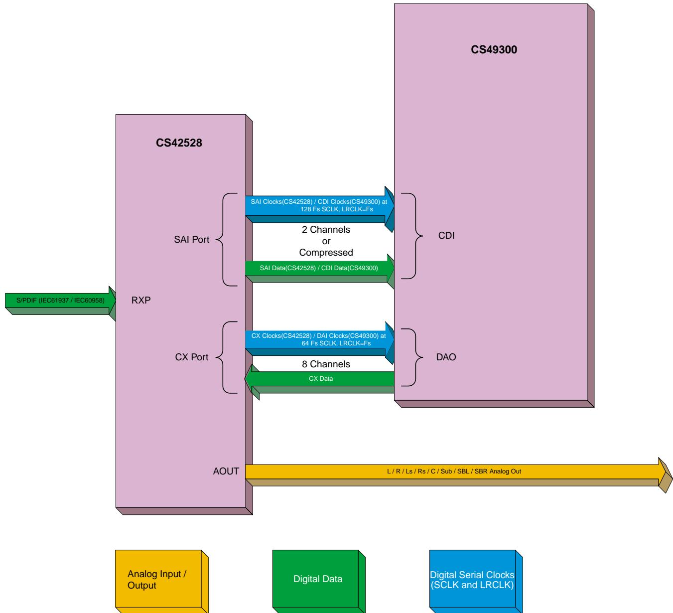
**Figure 5. Clock and Data Connections for S/PDIF (IEC61937 / IEC60958) Input**
