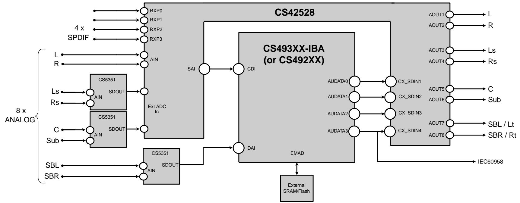
**Figure 1. Block Diagram of the CRD42528**
