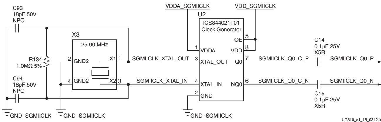
Figure 1-17: Ethernet 125 MHz SGMII GTX Clock
