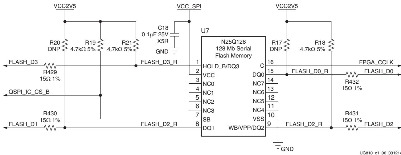
Figure 1-6: 128 Mb Quad SPI Flash Memory
