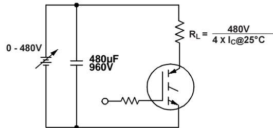
**Fig. 13b** - Pulsed Collector Current Test Circuit
