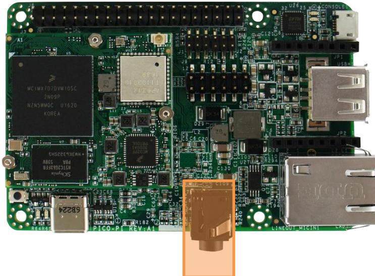
**Figure 15 - PICO-PI-IMX7 Audio I<sup>2</sup>S Signal Location**
