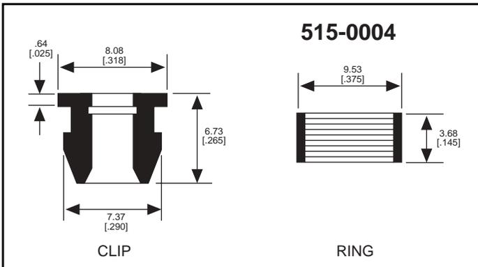
515-0004 Snap-In Mounting Clips for use with the following LEDs:
