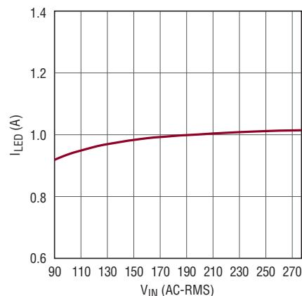
Figure 3. I<sub>OUT</sub> vs Input Voltage
