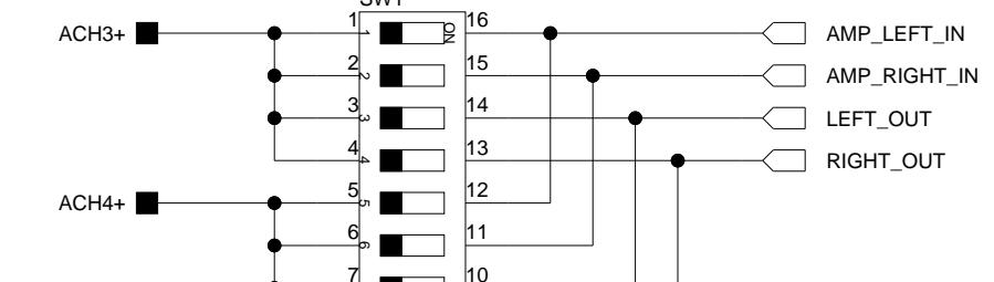
SW1: Oscilloscope Select Switch
