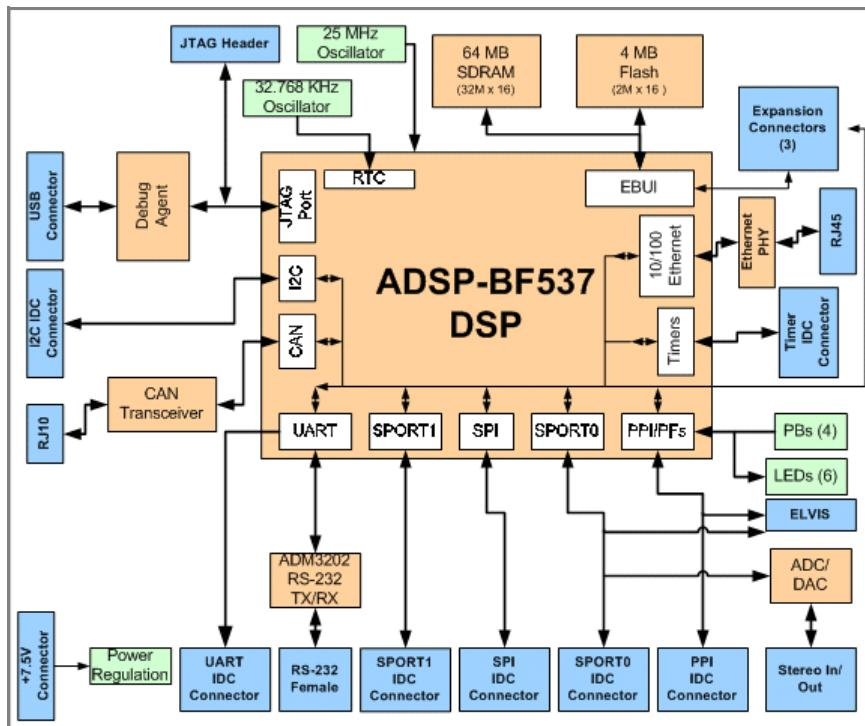
Figure 2-1. System Architecture
