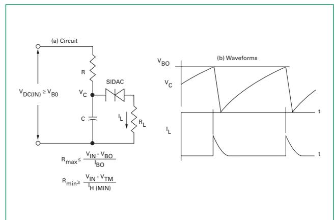
**Figure 15: Low-voltage Input Circuit for Gas Ignition**
