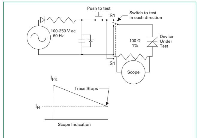
**Figure 13: Basic SIDAC Circuit**
