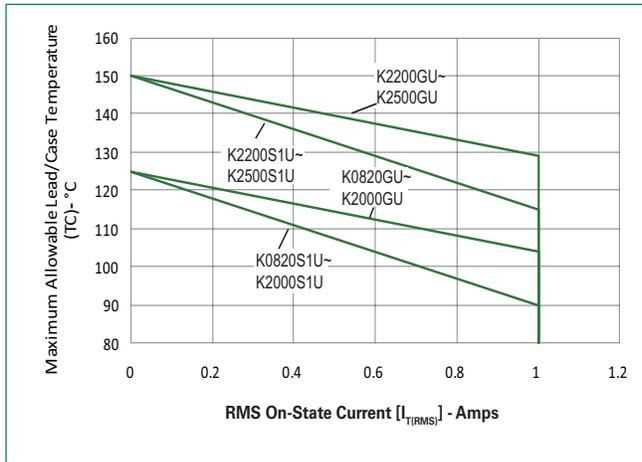
**Figure 10: Maximum Allowable Ambient Temperature vs. RMS On-State Current**
