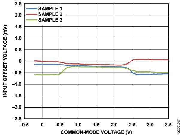
Figure 7. Input Offset Voltage ( $V_{os}$ ) vs. Common-Mode Voltage ( $V_{cm}$ ),
