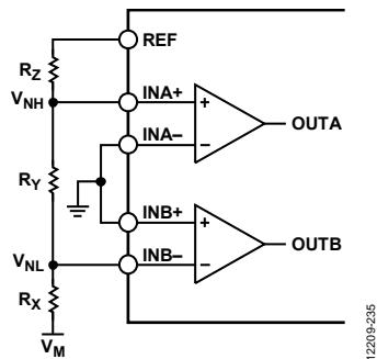
Figure 35. Negative Undervoltage/Ovvoltage Monitoring Configuration
