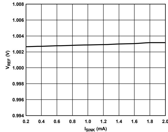
Figure 28. Reference Voltage ( $V_{REF}$ ) vs. Sink Current ( $I_{SINK}$ ) of the REF Pin,
