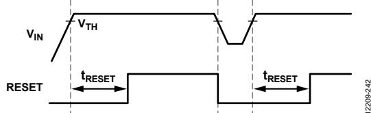
Figure 42. Threshold and Timeout Programmable Voltage Supervisor Timing Diagram
