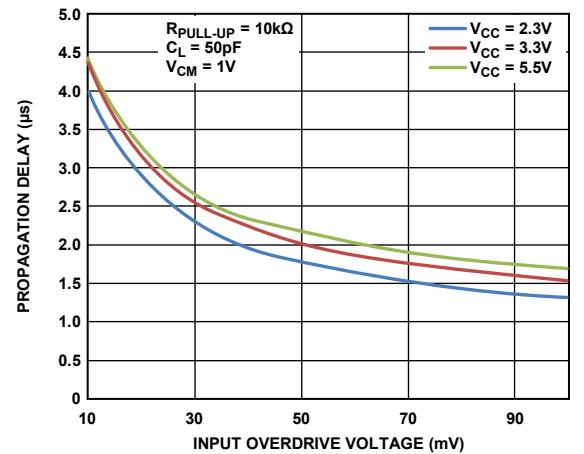
Figure 23. Propagation Delay vs. Input Overdrive Voltage, High to Low, Channel B
