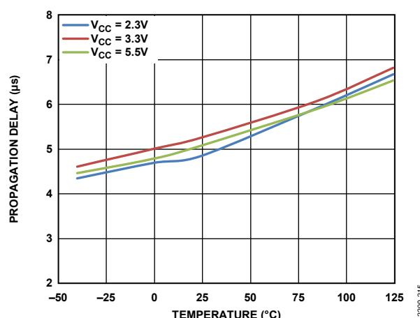
Figure 15. Propagation Delay vs. Temperature, Low to High,  $V_{OD} = 10 mV$
