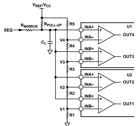
Figure 39. Circuit Configuration for a Mirrored Voltage Sequencer
