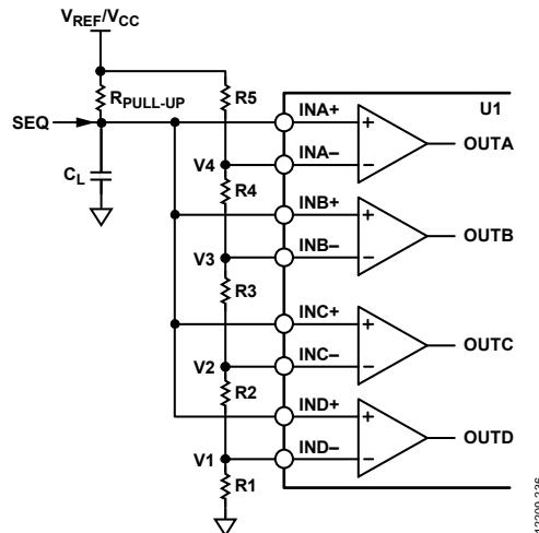
Figure 36. Programmable Sequencing Control Circuit
