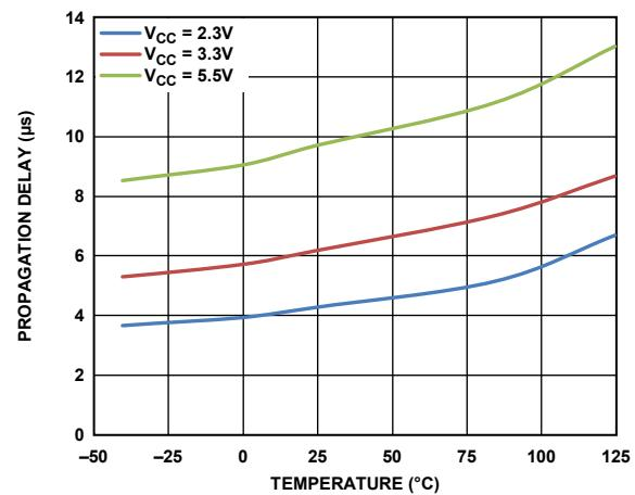
Figure 18. Propagation Delay vs. Temperature, High to Low,  $V_{OD} = 10 mV$
