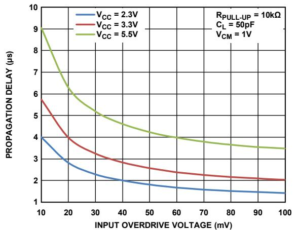
Figure 22. Propagation Delay vs. Input Overdrive Voltage, High to Low
