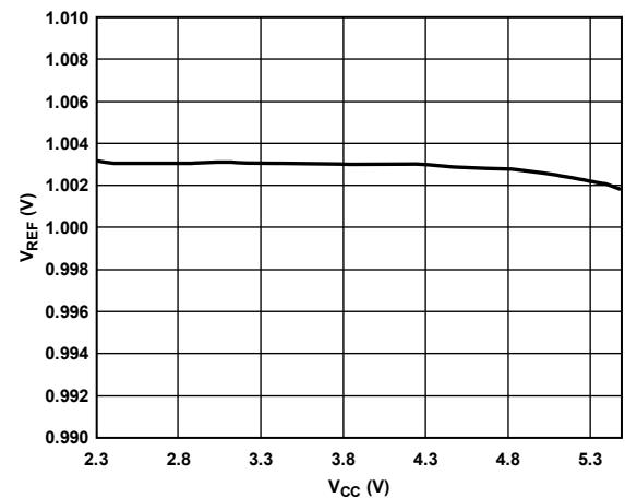
Figure 29. Reference Voltage ( $V_{REF}$ ) vs. Supply Voltage ( $V_{CC}$ )
