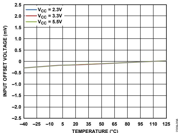
Figure 8. Input Offset Voltage ( $V_{os}$ ) vs. Temperature for
