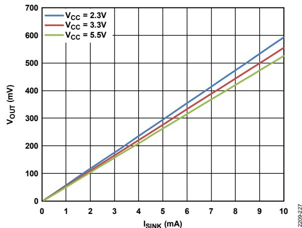
Figure 27. Output Voltage ( $V_{OUT}$ ) Low vs. Sink Current ( $I_{SINK}$ ) for
