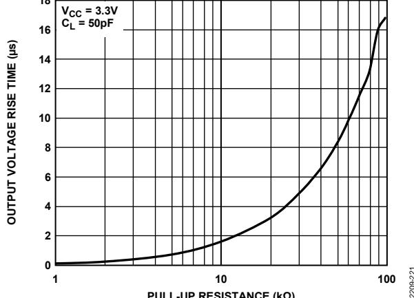
Figure 21. Output Voltage Rise Time ( $t_R$ ) vs. Pull-Up Resistance ( $R_{PULLUP}$ )
