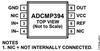
Figure 4. ADCMP394 Pin Configuration
