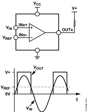
Figure 31. Basic Comparator and Input and Output Signals
