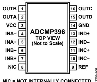
Figure 6. *ADCMP396 Pin Configuration*Table 6. *ADCMP396 Pin Function Descriptions*
