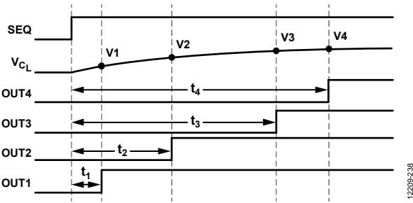
Figure 38. Programmable Sequencing Control Circuit Timing Diagram
