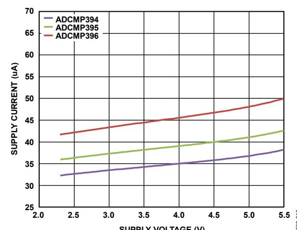
Figure 12. Supply Current ( $I_{cc}$ ) vs. Supply Voltage ( $V_{cc}$ ) at Output High
