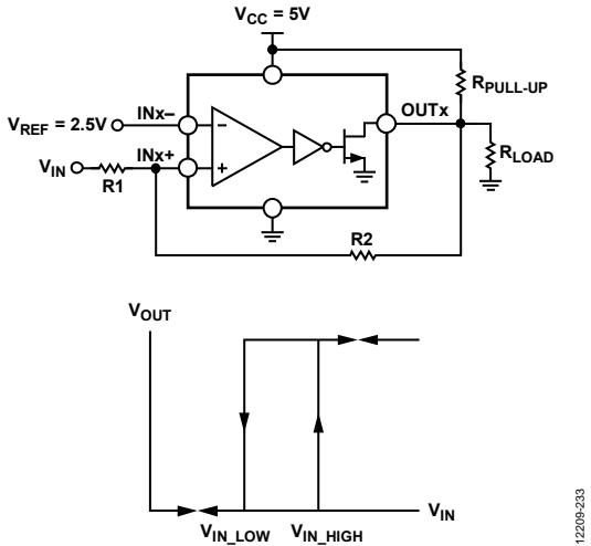
Figure 33. Noninverting Comparator Configuration with Hysteresis
