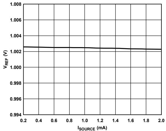
Figure 25. Reference Voltage ( $V_{REF}$ ) vs. Source Current ( $I_{SOURCE}$ ) of the REF Pin,
