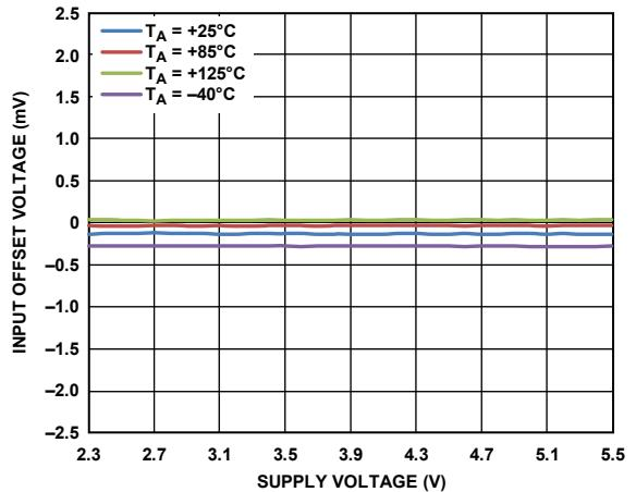
Figure 10. Input Offset Voltage ( $V_{os}$ ) vs. Supply Voltage ( $V_{cc}$ ),  $V_{cm} = 1\text{ V}$
