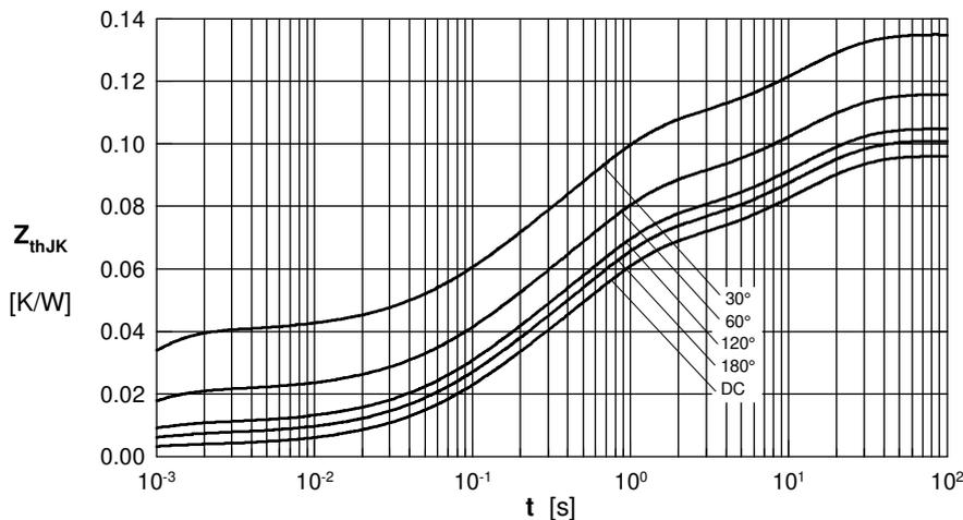
Fig. 8 Transient thermal impedance junction to heatsink
