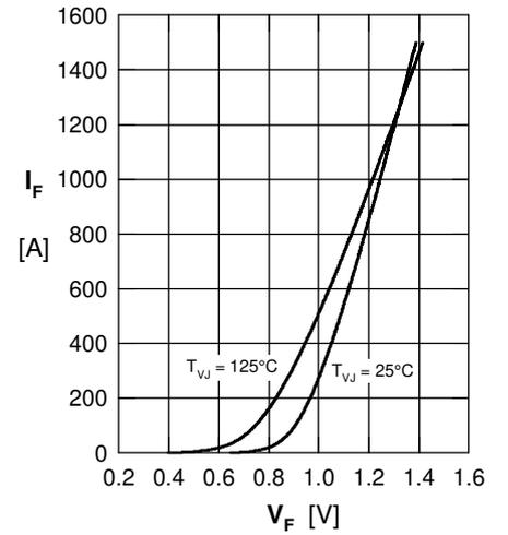
Fig. 5 Forward current  $I_F$  versus  $V_F$
