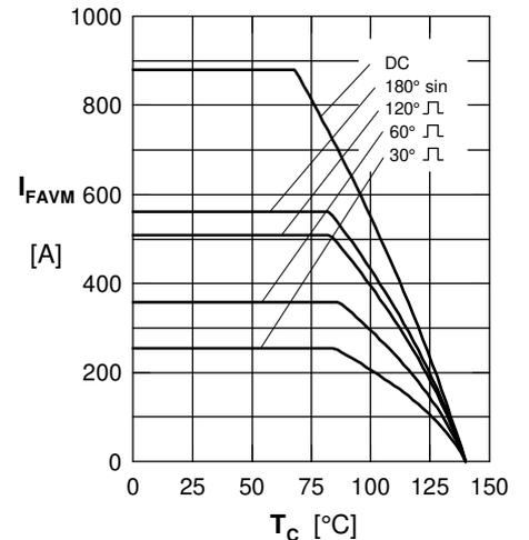
Fig. 3 Maximum forward current at case temperature
